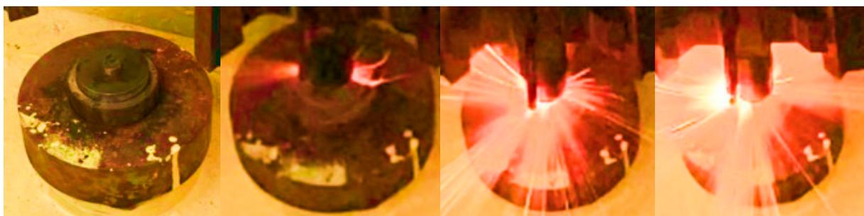
**Figure 13.** Reactions developed by the composite formulations during impact tests.
