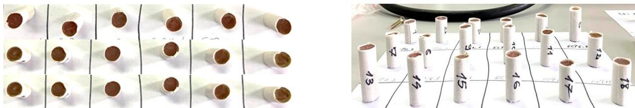
**Figure 8.** Cylindrical grain propellant molds.
