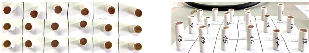
**Figure 8.** Cylindrical grain propellant molds.
