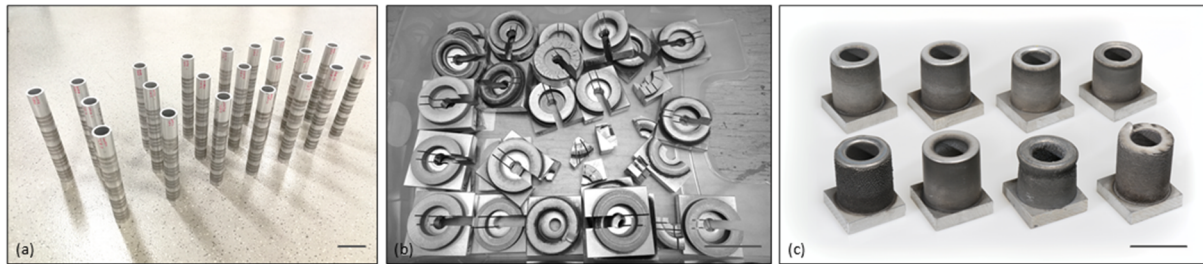
Figure 5. Exterior views of specimens of (a) single tracks, (b) 3D-parts with about 5 mm height and used for hardness tests, and (c) 3D-parts with about 50 mm height and used for tensile tests. The black bars indicate a length of 50 mm.
