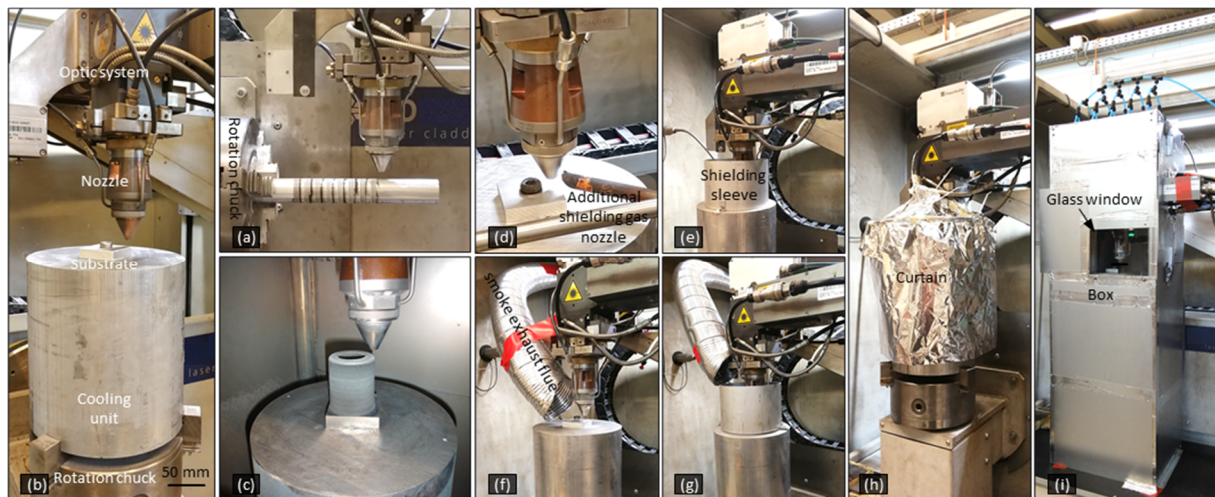
Figure 4. Photos of the basic experimental setup for fabricating (a) single tracks and (b) 3D-parts “Or”. Most of the 3D-parts like that shown in (c) were made with additional shielding concepts: (d) an additional shielding gas flow “Ad”, (e) a shielding sleeve “Ri”, (f) a smoke exhaust flue “Ex”, (g) a combination of the sleeve and the flue “RE”, (h) an Al curtain “Fo”, and (i) a protective box “Bo”. The designators in quotation marks are the short forms used in Table 1. “Bo” has a larger interior space and is thus more heat resistant than “Fo”. The letters in quotation marks are specimen designations (see Table 1).
