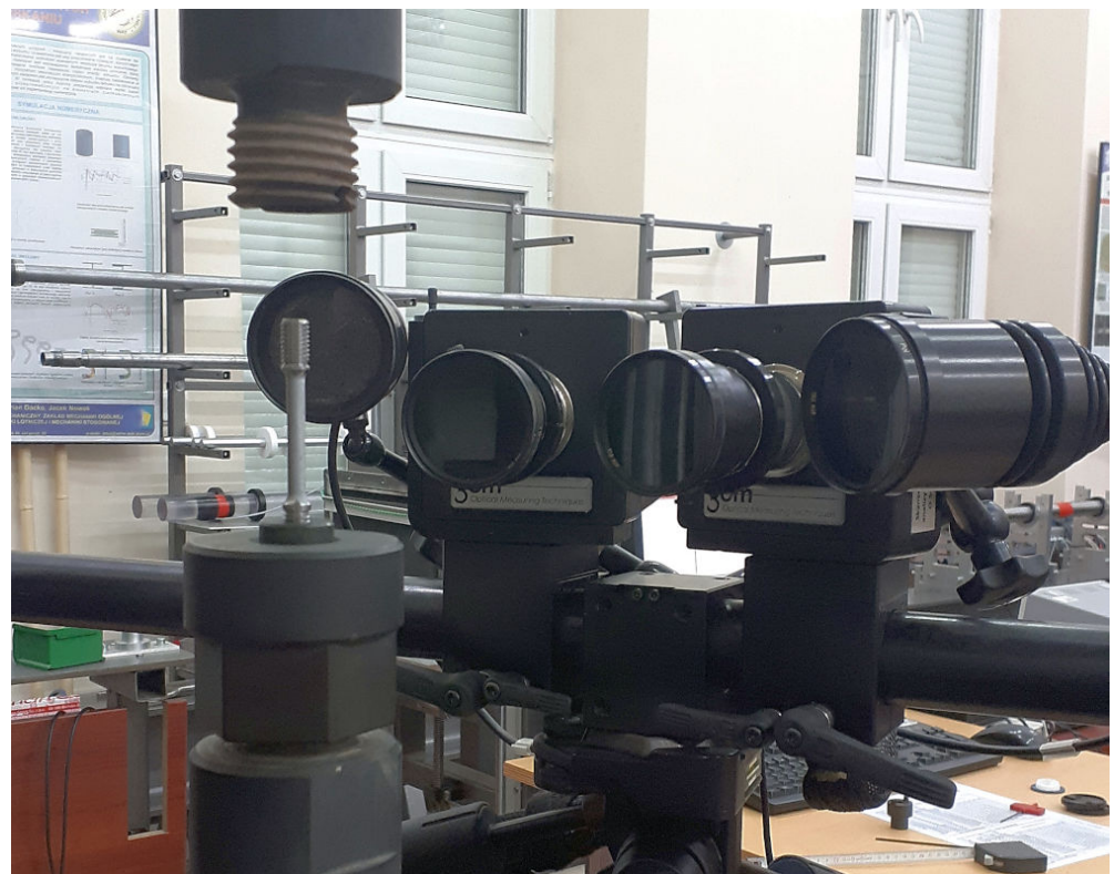
Figure 4. Installation of an exemplary specimen in a threaded holder of the Instron 8862 machine along with the setup of the 3D cameras of the DIC measurement system.
