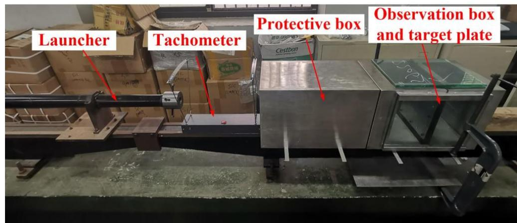
**Figure 10.** Harpoon impact test layout.
