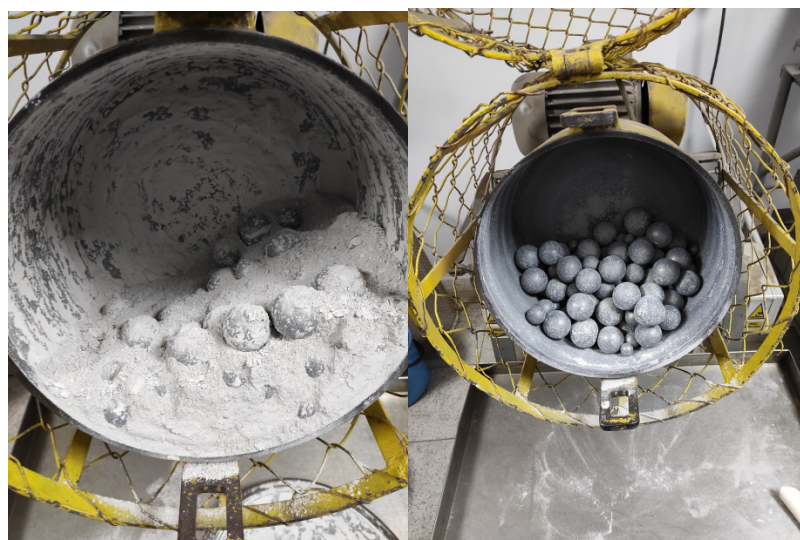
Figure 1. Ball mill-laboratory scale.
