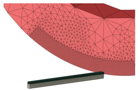
Figure 2. Undeformed mesh for cutting tool and workpiece.
