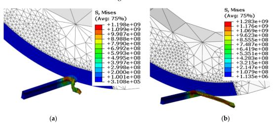
**Figure 4.** Chip formation and von-Mises-stress contours for SPRT and workpiece at different feed rates: (a) f = 0.1 mm/rev, (b) f = 0.2 mm/rev (V = 80 m/min, d = 0.3 mm and i = 17°).
