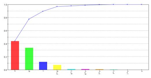
Figure 9. Specific-cutting-energy dependencies on input variables and their interactions.
