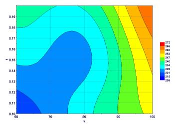
Figure 11. Combined effect of cutting speed and feed rate on maximum tool temperature.
