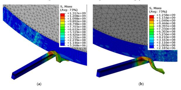
**Figure 5.** Chip formation and von-Mises-stress contours for SPRT and workpiece at different inclination angles: (a)  $i = 9^{\circ}$ , (b)  $i = 25^{\circ}$  (V = 100 m/min, f = 0.1 mm/rev, d = 0.3 mm).
