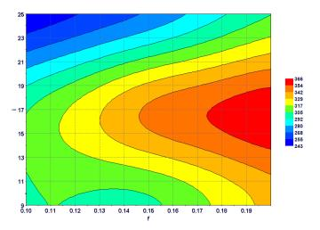
Figure 10. Combined effect of feed rate and inclination angle on maximum tool stress.
