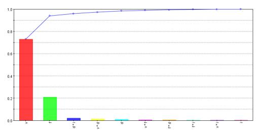
Figure 8. Tool-temperature dependencies on input variables and their interactions.
