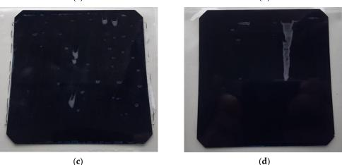
**Figure 3.** Laminated solar cells: (**a**) without defects; (**b**) adhesive stains on the surface caused by too fast feed; (**c**,**d**) damp patches from the adhesive caused by too low temperature of lamination.
