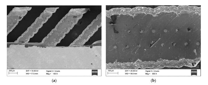
**Figure 8.** Topography of the electric contact surfaces of a monocrystalline silicon photovoltaic cell of the N-type: (**a**) contact of fingers (grid lines) with connectors; (**b**) finger (grid line).
