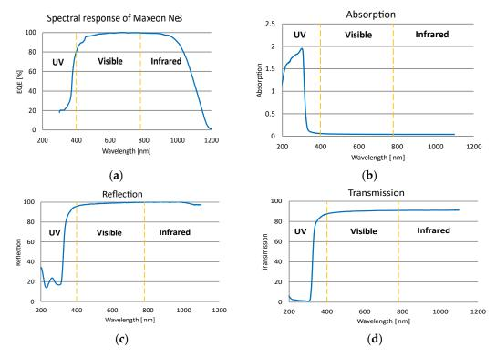
**Figure 5.** Characteristics of: (a) spectral response of Maxeon Ne3; (b) 100  $\mu$ m film absorption; (c) 100  $\mu$ m film reflection; (d) 100  $\mu$ m film transmission.
