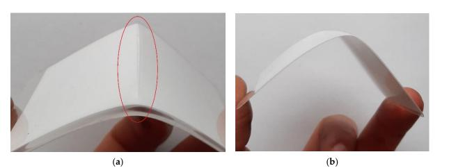
**Figure 2.** Samples tests: (a) incision test of a film with a thickness of 250  $\mu$ m with a burst gap; (b) incision test of a film with a thickness of 100  $\mu$ m, which does not enlarge the damage.
