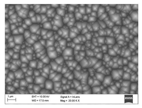
Figure 6. SEM textured surface topography of the N-type monocrystalline silicon solar cell.
