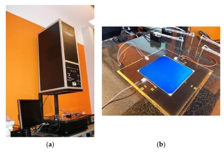
**Figure 4.** Test stand: (**a**) solar simulator with a xenon flash lamp, measuring table, and computer for downloading current–voltage characteristics; (**b**) research conducted on flexible solar cells placed on the measuring table.
