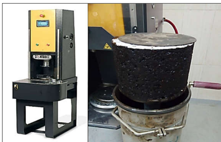
Figure 4. Asphalt sample compacted using SGC.
