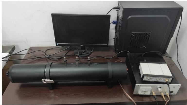
**Figure 9.** Sound absorption coefficient test equipment.
