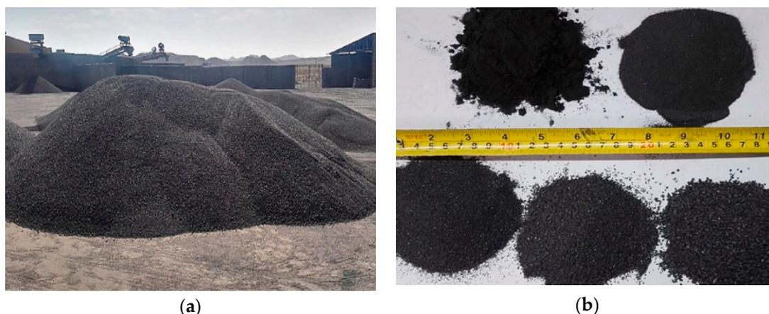
**Figure 2.** Pictures of CS: (a) before grinding; (b) after grinding [47].
