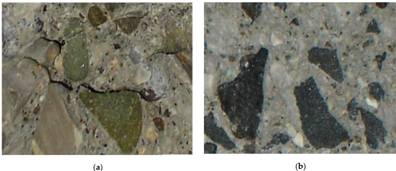
**Figure 11.** Failure sections of concrete with different coarse aggregates: (a) limestone coarse aggregate; (b) CS coarse aggregate [30].
