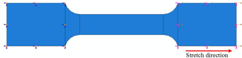
**Figure 10.** ABAQUS simulation model's boundary conditions.
