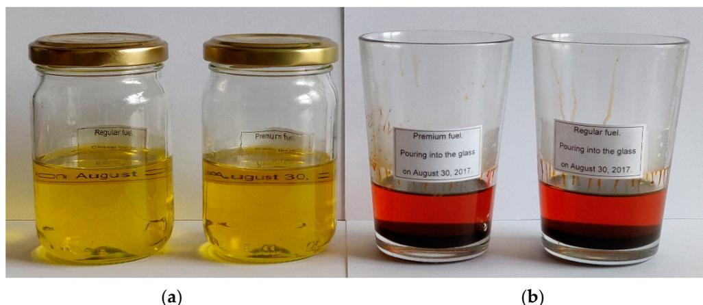
**Figure 2.** Premium and regular fuels stored in an optical darkroom for five years: (a) in closed jars; (b) in open glasses.
