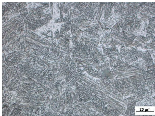
**Figure 9.** Microstructure of HAZ of welded joint exposed to temperature 1100 °C.
