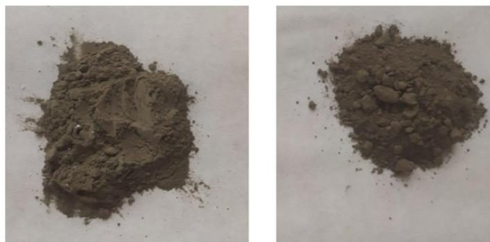
Figure 1. Fly ash (right) and titanium dioxide waste (left).
