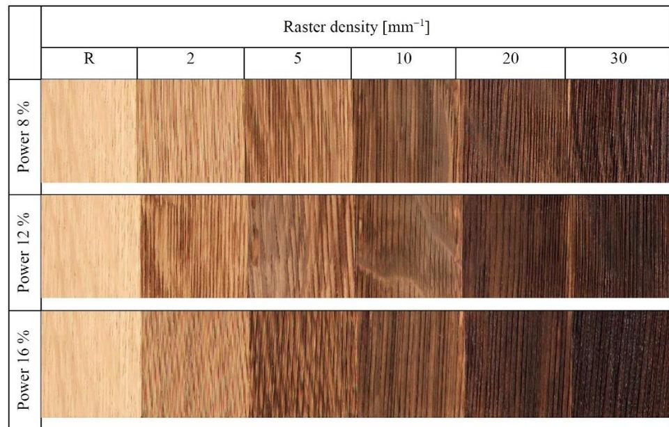
**Figure 10.** Oak wood surface treated with CO<sub>2</sub> laser.
