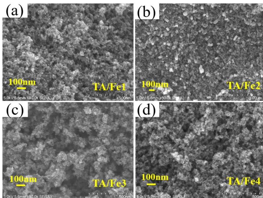
Figure 5. FESEM images of the Fe-doped titanium oxide-based aerogel catalysts.
