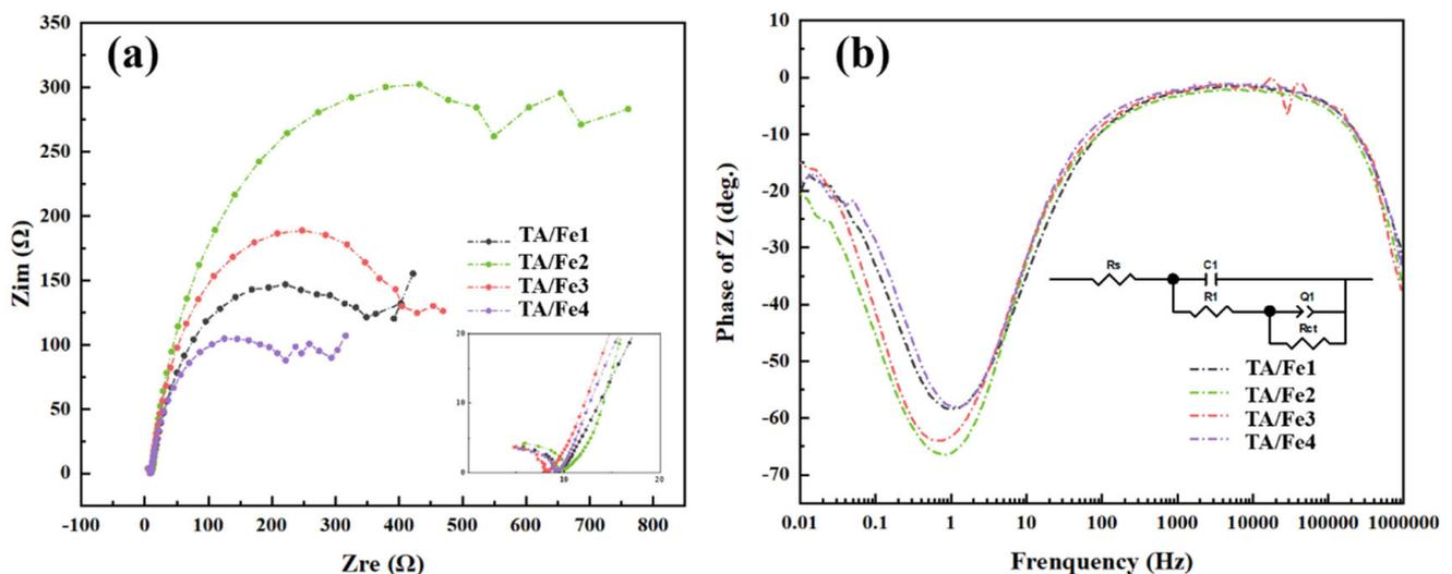
**Figure 12.** (a) Nyquist plots and (b) Bode diagrams of the titanium oxide-based aerogel catalysts doped by different Fe sources.
