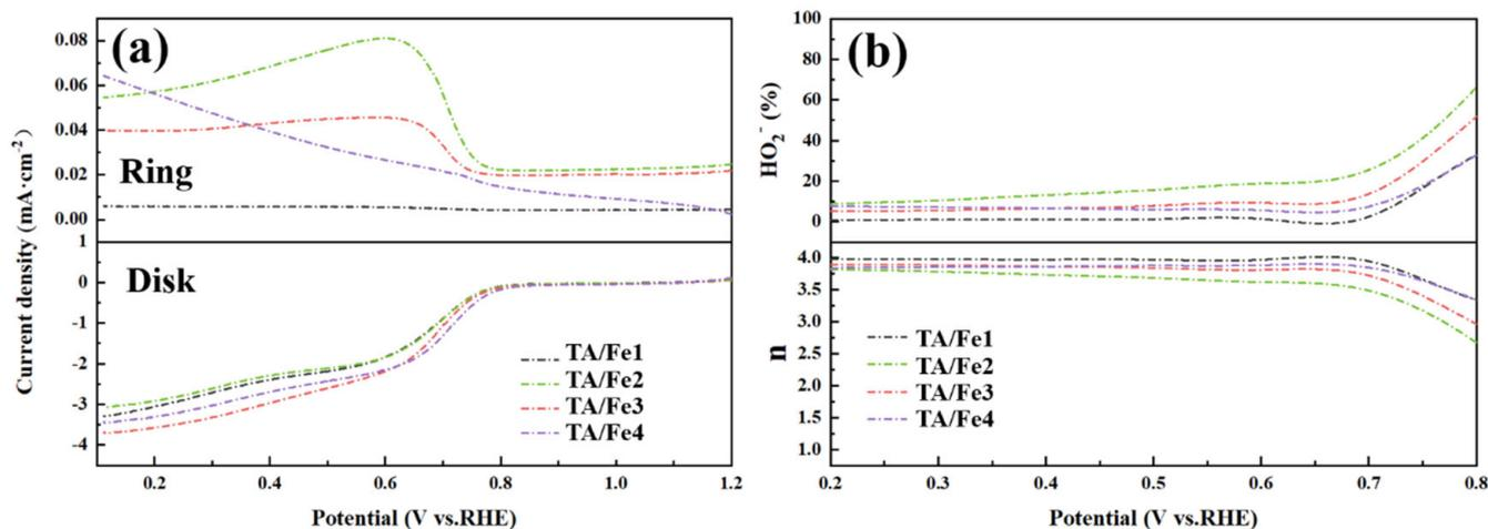
**Figure 11.** (a) Potentiostatic polarization curves and (b) hydrogen peroxide yields and transfer number of the as-prepared aerogel catalysts (at the constant voltage of 1.3 V vs. RHE).
