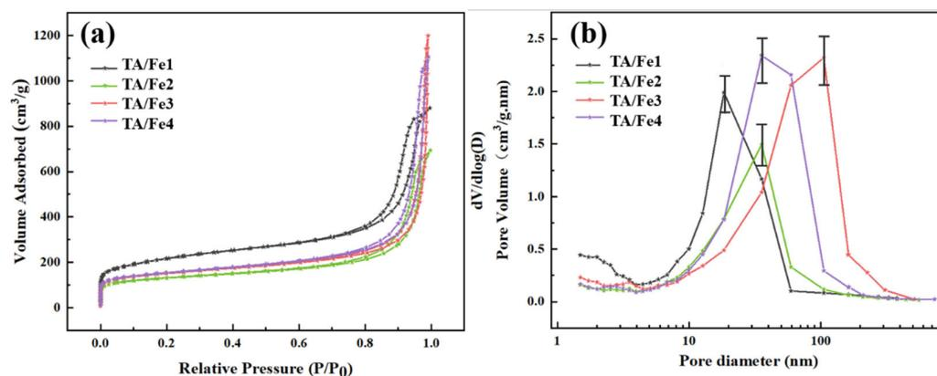
**Figure 4.** (a)  $N_2$  adsorption/desorption curves and (b) pore size distribution of the TA/Fe1, TA/Fe2, TA/Fe3, and TA/Fe4.
