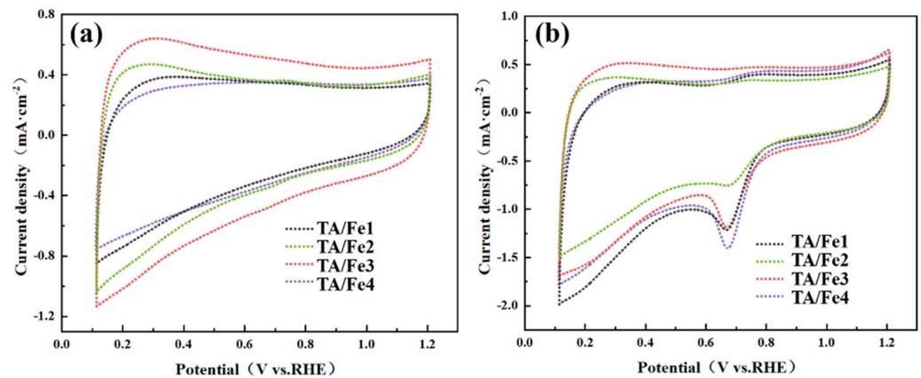
**Figure 8.** CV curves of the titanium oxide-based aerogel catalysts doped by different Fe sources: (a)  $N_2$  test condition, (b)  $O_2$  test condition.
