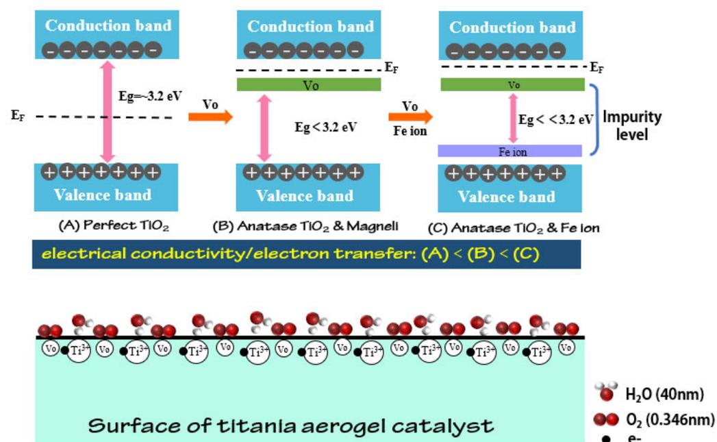
**Figure 13.** The influence mechanism of the oxygen vacancies, doping effect, and pore structure.
