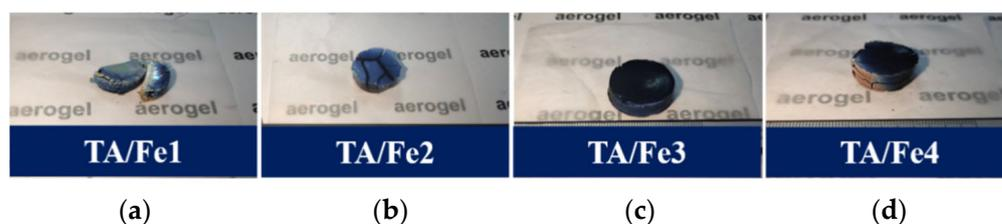
**Figure 2.** Photographs of TA/Fe<sub>s</sub>: (a) doped by Fe(NO<sub>3</sub>)<sub>3</sub>·9 H<sub>2</sub>O, (b) doped by C<sub>15</sub>H<sub>21</sub>FeO<sub>6</sub>, (c) doped by K<sub>4</sub>Fe(CN)<sub>6</sub>·3H<sub>2</sub>O, and (d) doped by Fe<sub>3</sub>O<sub>4</sub>.
