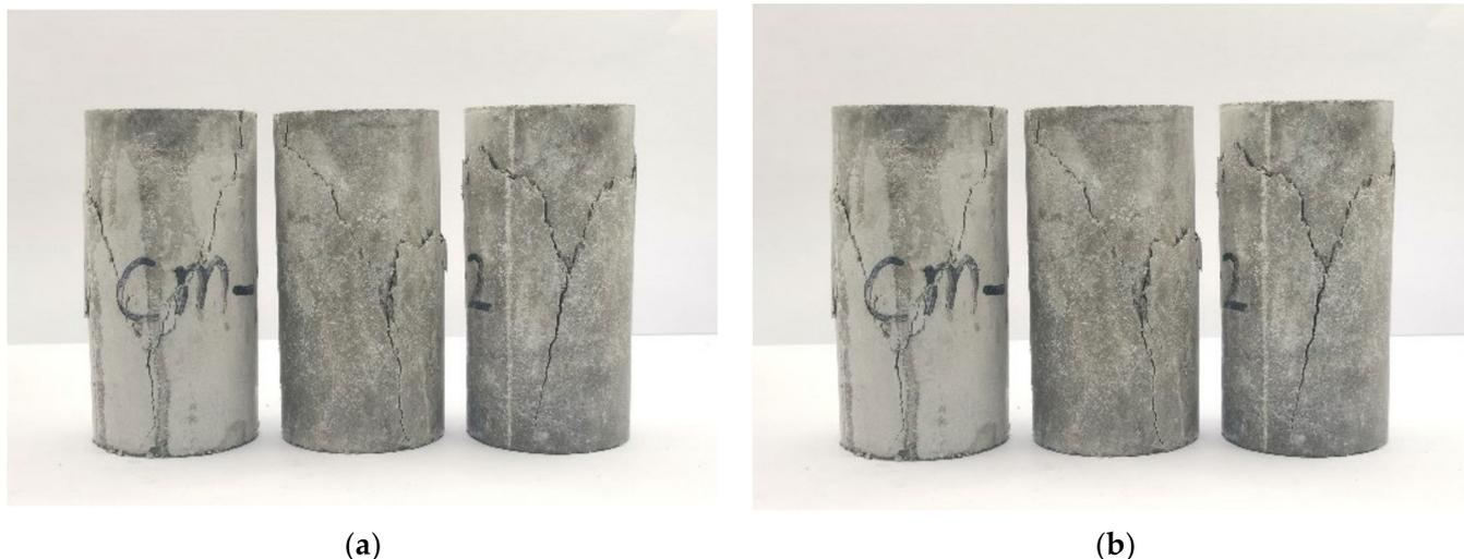
**Figure 5.** Failure patterns of specimens: (a) uniaxial monotonic compression tests; (b) uniaxial cyclic loading and unloading tests.
