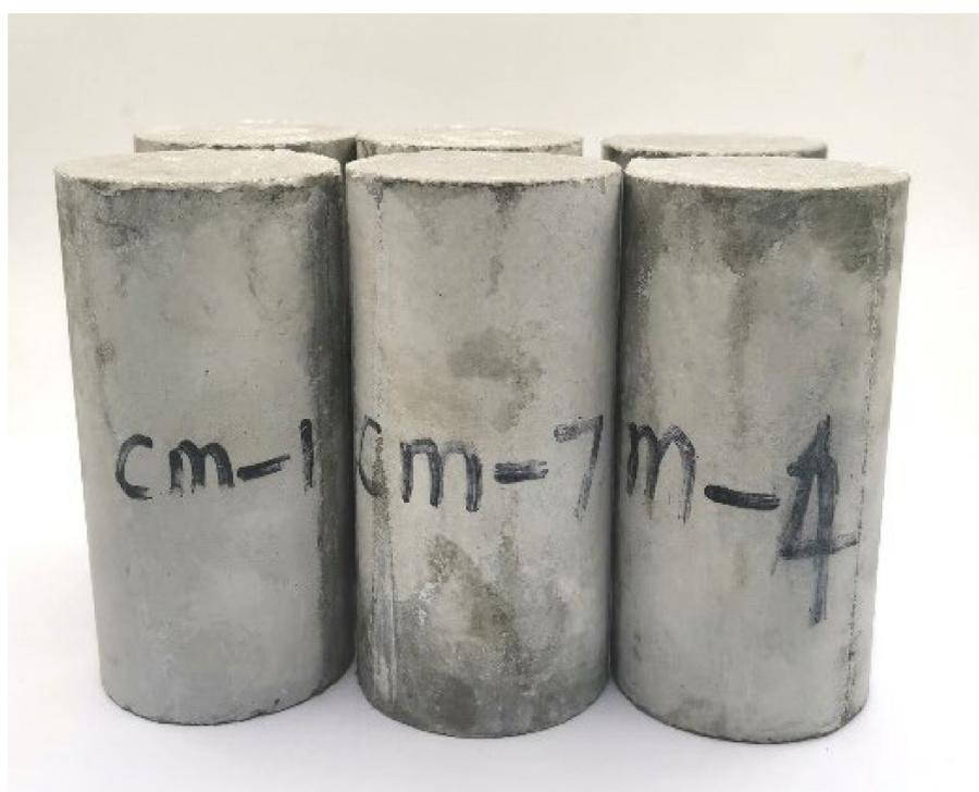
**Figure 1.** Cement mortar specimens for mechanical testing.
