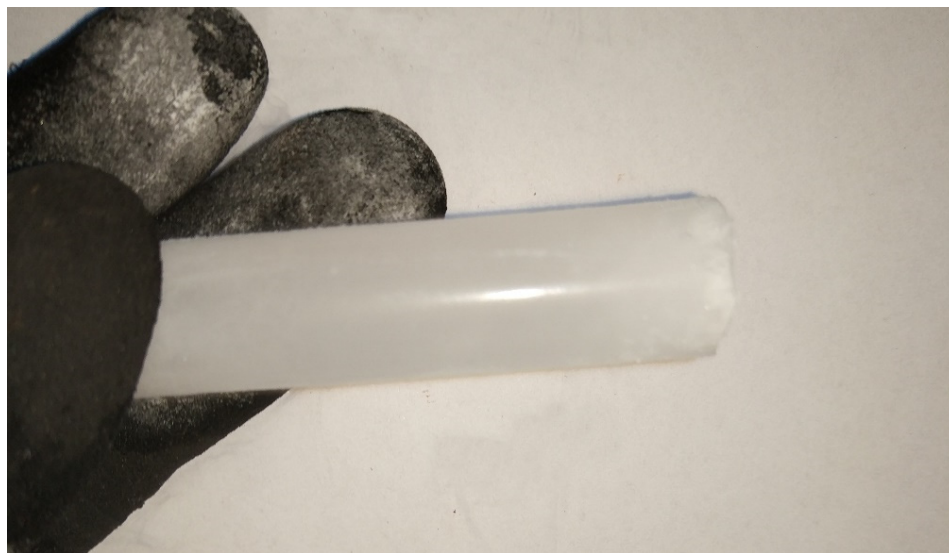
Figure 10. Sample of extruded material of uniform appearance and uniform density distribution.
