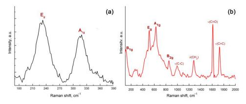
**Figure 6.** Raman spectra of  $SnS_2$  (**a**) and 2D  $SnO_2$  (**b**) samples.
