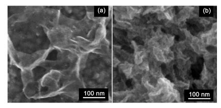
Figure 4. SEM images of SnS<sub>2</sub> nanosheets before (**a**) and after (**b**) oxidation at 500 °C.
