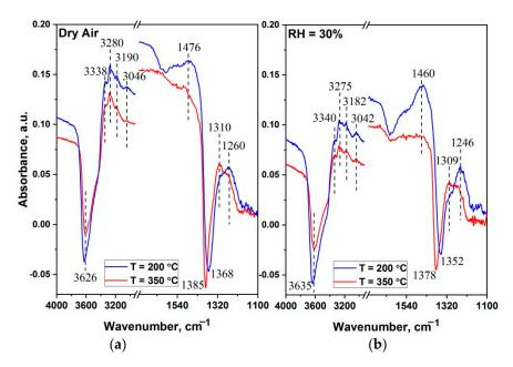
**Figure 11.** In situ DRIFT spectra of 2D SnO<sub>2</sub> (**a**) in dry (RH<sub>25</sub> = 0%) and (**b**) in humid (RH<sub>25</sub> = 30%) air containing 100 ppm NH<sub>3</sub> at temperatures of 200 °C (blue line) and 350 °C (red line).
