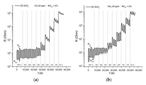
**Figure 9.** Temperature dependencies of the dynamic-sensor response of  $2D \text{ SnO}_2$  when detecting 20 ppm CO (**a**) and 20 ppm NH<sub>3</sub> (**b**) in dry air (RH<sub>25</sub> = 0%).
