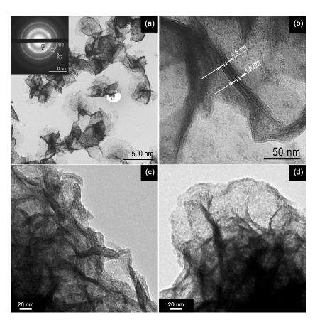
**Figure 3.** TEM images of  $SnS_2$  nanosheets before (**a**–**c**) and after (**d**) oxidation at 500 °C. Inset shows the electron-diffraction pattern.
