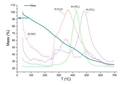
**Figure 1.** TG curve and temperature dependencies of ionic current for m/z = 18 (H<sub>2</sub>O), 30 (NO), 44 (CO<sub>2</sub>), 64 (SO<sub>2</sub>) for SnS<sub>2</sub> oxidation in air.
