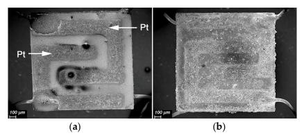
**Figure 2.** SEM image of alumina substrate with Pt contacts: (**a**) bare substrate, (**b**) covered with 2D SnO<sub>2</sub>.
