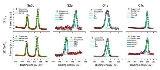
Figure 7. XP-spectra of SnS<sub>2</sub> and 2D SnO<sub>2</sub>.
