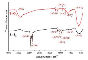
Figure 8. FTIR spectra of SnS<sub>2</sub> and 2D SnO<sub>2</sub> samples.
