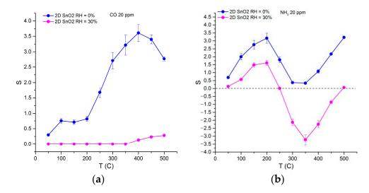
**Figure 10.** Temperature dependencies of 2D SnO<sub>2</sub> sensor response when detecting 20 ppm CO (**a**) and 20 ppm NH<sub>3</sub> (**b**) in dry (RH<sub>25</sub> = 0%) and humid (RH<sub>25</sub> = 30%) air.
