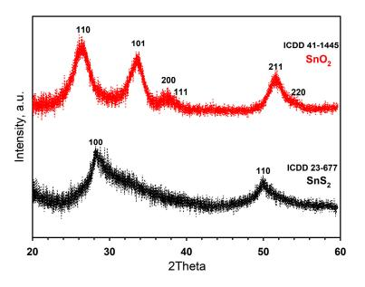
Figure 5. X-ray diffraction patterns of SnS<sub>2</sub> nanosheets and 2D SnO<sub>2</sub> powder.
