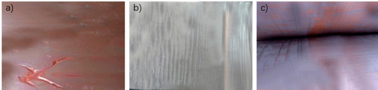
**Figure 12.** Casting and rolling of copper and aluminum at different casting speeds at pouring temperature of 700 °C. (a) 1.1 m/min; (b) 1.2 m/min; (c) 1.3 m/min.
