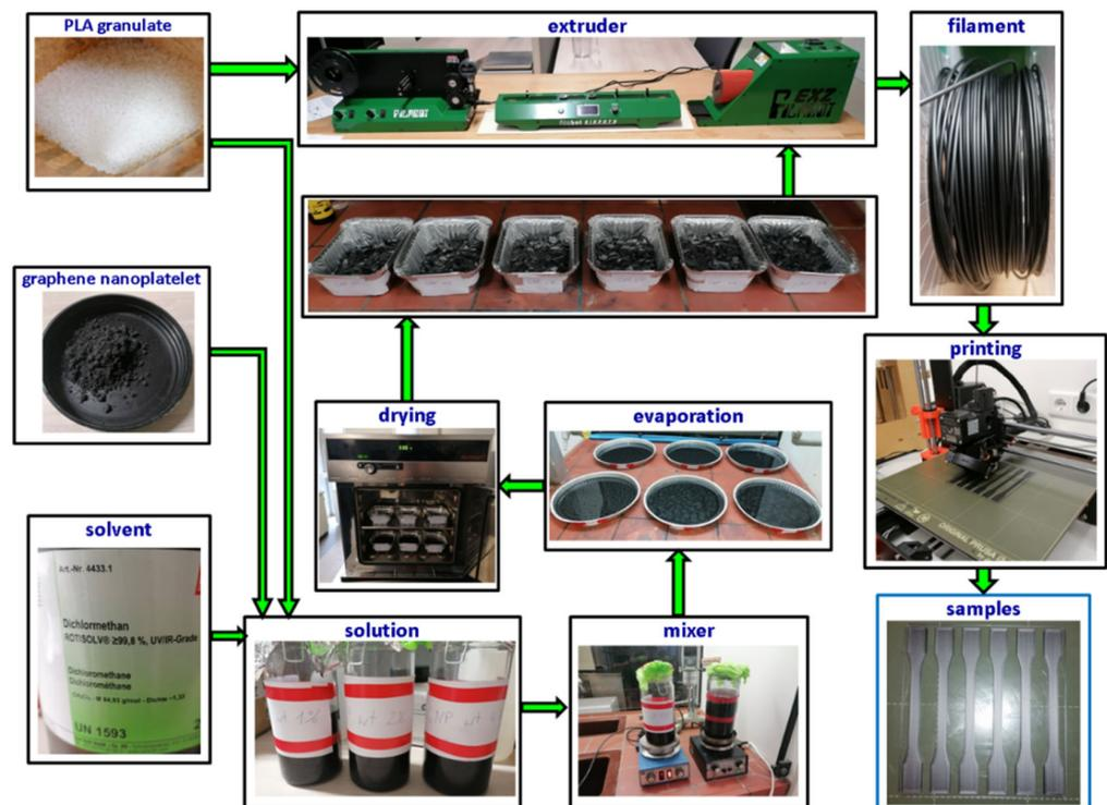
**Figure 1.** Schematic course of preparing printed samples made of pure PLA and PLA with GNP.
