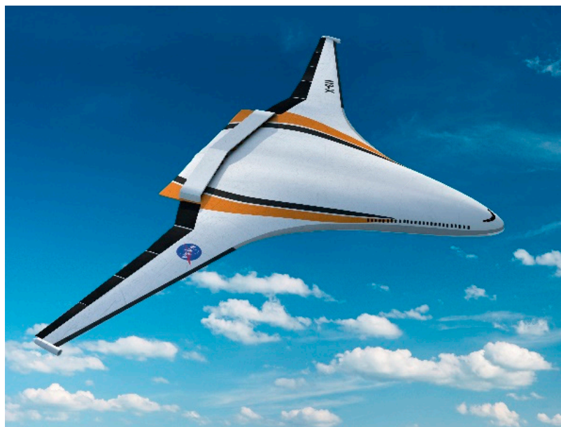
Figure 2. NASA's N3-X, Turboelectric blended wing body concept.
