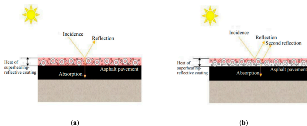
Figure 8. Working principle of coatings with different structures. (a) Single-layer coating structure, (b) Double-layer coating structure.
