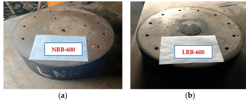
**Figure 1.** Test specimen of the two rubber bearings: (a) NRB-600 specimen; (b) LRB-600 specimen.
