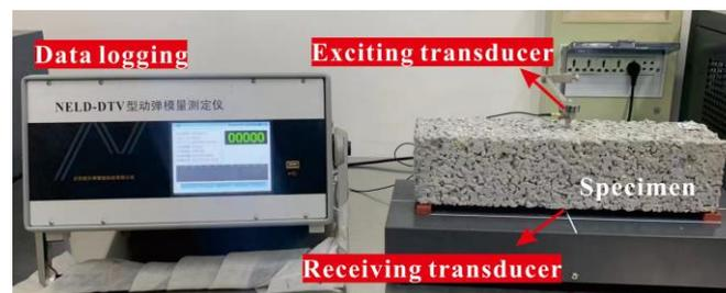
**Figure 5.** Test setup for dynamic elasticity modulus.
