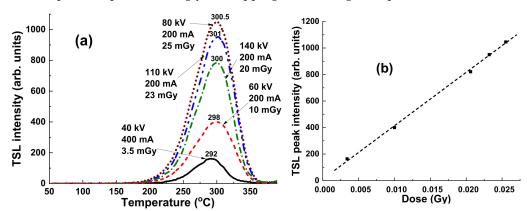
**Figure 9.** (a) Dependence of TSL peak intensity and peak position for YAG:Ce crystal sample on irradiation dose by continuous X-ray photons working with NAP in the 40–140 KV range and current in the 200–400 mA range; (b) TSL intensity as a function of the dose of irradiation for the YAG:Ce crystal detector.
