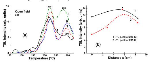
**Figure 13.** (a) TSL glow curves for YAG:Ce crystal detector irradiated by 15 MV X-ray photons from a Clinac 2300 accelerator in open field mode; (b) dependence of the intensity of two TSL peaks of YAG:Ce crystal at 220  $^{\circ}$ C (1) and 285  $^{\circ}$ C (2) on the distance x between sample and centers of target.
