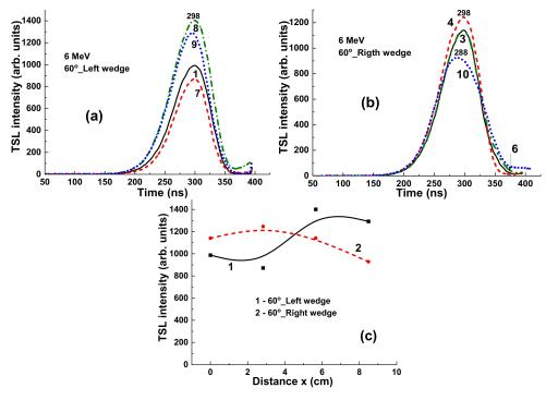
**Figure 14.** (**a**,**b**) TSL glow curves for YAG:Ce crystal detectors irradiated by 15 MV X-ray photons from a Clinac 2300 accelerator in the case of using additional wedges 60o\_Left (**a**) and 60o\_R-right (**b**); (**c**) dependence of the intensity of TSL peaks on distance x between sample and center of target (see Figures 1 and 9).
