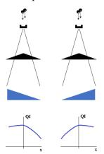
Figure 8. Effect of simultaneous work of flattening filter and hard wedge for both wedge orientations.
