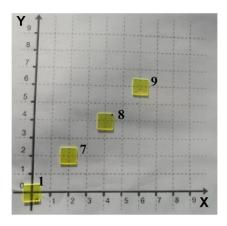
**Figure 1.** The position of the samples on the table of Clinac 2300CD Silhouette (Varian Medical Systems, Palo Alto, CA, USA) accelerator relative to the center of target (**left side**) and the position of the YAG:Ce detectors on the experimental x-y plane (**right side**). The positions of the detectors are also identified by numbers in the x-y plane of the right figure.
