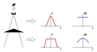
**Figure 6.** High energy X-ray (6 MV and 15 MV) intensity (I) and radiation quality (QI) off-axis characteristics at selected stages of therapeutic beam generation in a classic medical accelerator—simplification.
