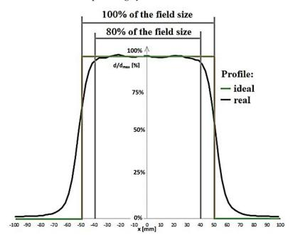
Figure 4. Typical beam profile for radiotherapeutic applications.
