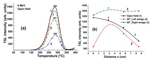
**Figure 10.** (a) TSL glow curves for YAG:Ce crystal samples irradiated by 6 MV X-ray photons from a Clinac 2300 accelerator in open field mode; (b) dependence of intensity of TSL peaks on the distance x between sample and centers of target (see Figure 1).
