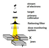
Figure 5. Diagram of the beam collimation system in a standard medical accelerator—Linac head.
