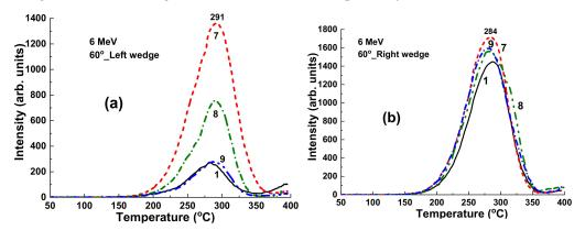
**Figure 11.** (a) TSL glow curves for YAG:Ce crystal samples irradiated by 6 MV X-ray photons from Clinac 2300 accelerator in the case of using additional  $60^{\circ}$ \_Left (a) and  $60^{\circ}$ \_Right (b) wedges (see Figure 8).
