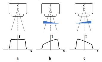
**Figure 7.** Influence of wedge filter on beam intensity distribution: (a) open field (no wedge), (b) left side wedge orientation, (c) right side wedge orientation.
