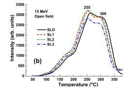
**Figure 15.** (a) Position of LuAG:Ce crystal samples on the experimental x-y plane. (b) TSL glow curves for set of LuAG:Ce crystal detectors irradiated by 15 MV X-ray photons from a Clinac 2300 accelerator in the open field mode.
