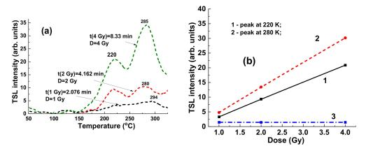
**Figure 12.** (a) Dependence of intensity of TSL glow curves for YAG:Ce crystal detector on the dose of irradiation by  $^{60}$ Co source; (b) intensity of TSL glow peaks of YAG:Ce crystal at 220 °C (1) and 285 °C (2) source and  $I_{285}/I_{220}$  ratio of intensity of these peaks (3) on dose of  $\gamma$  rays irradiation by  $^{60}$ Co.
