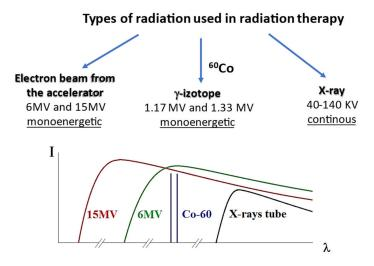
**Figure 3.** Different types of radiation used in this work (**top**); the schematic dependence of wavelength  $\lambda$  of X-rays on the type of radiation (**bottom**).
