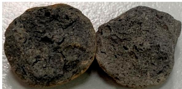
**Figure 1.** Appearance of lightweight expanded shale aggregates.
