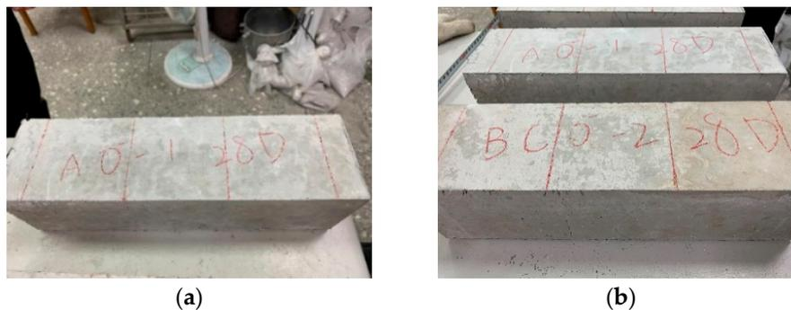
**Figure 21.** Destruction appearance of the concrete specimens after flexural test at room temperature: (a) control group; (b) experimental group.
