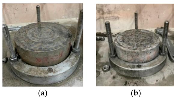
**Figure 26.** Appearance of the surface of the specimens exposed to high temperature after the water-penetration test: (a) control group; (b) experimental group.
