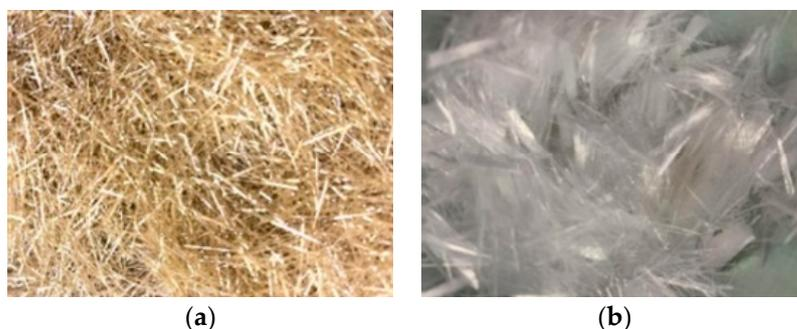
**Figure 2.** Fibers used in this study: (a) short micro-steel fibers; (b) polypropylene fibers.
