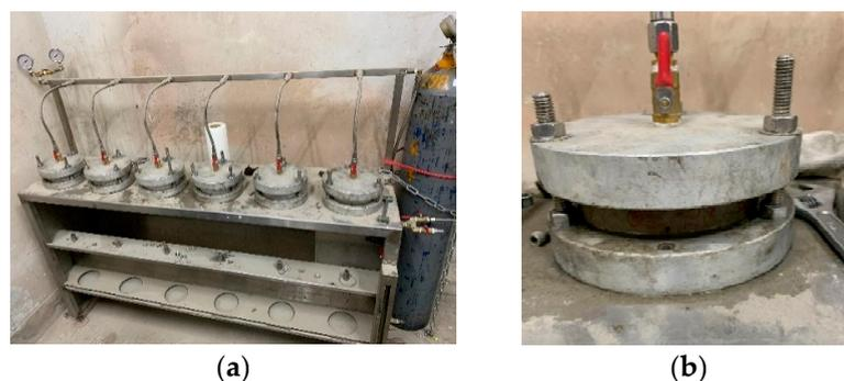
**Figure 7.** Water penetration test setup: (a) the case of six specimens; (b) the case of a single specimen.
