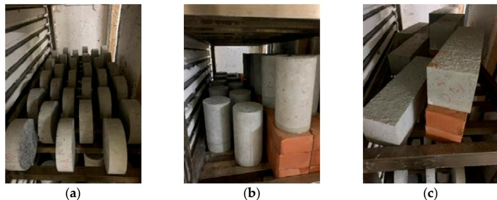
**Figure 5.** Configurations of specimens in high-temperature furnace: (a) water-penetration-test specimens; (b) compressive-strength-test specimens; (c) flexural-strength-test specimens.
