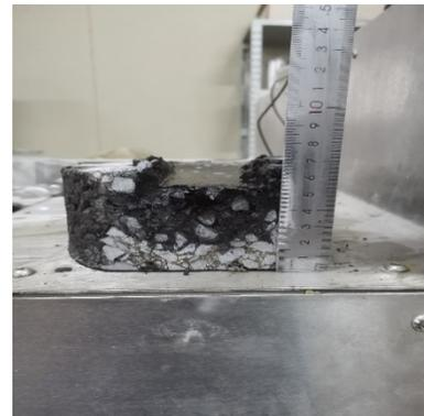
Figure 14. Specimen of HMPR-BF.
