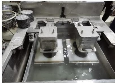
Figure 12. HWTT apparatus.
