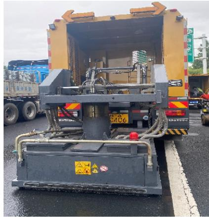
Figure 5. Pavement heating car.
