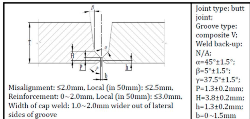
Figure 1. Design of composite V-groove.
