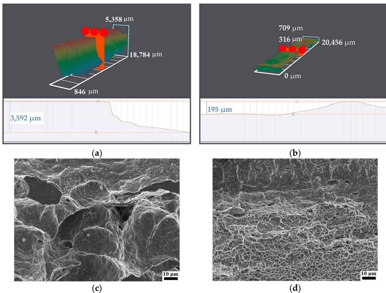
**Figure 9.** Contour map and fracture morphology of prefabricated fatigue crack tip under two heat input: (a,c) ultra-low heat input; (b,d) conventional heat input.
