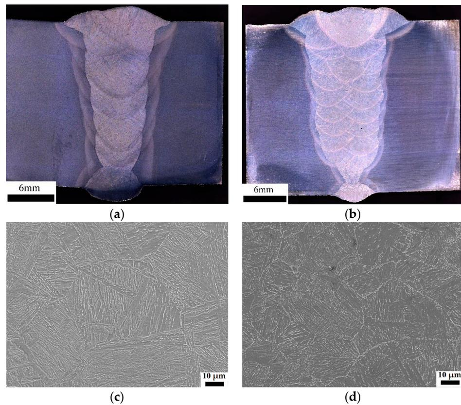
**Figure 2.** Macro-morphology of girth welded joints and microstructure of CGHAZs with different heat inputs: (a,c) conventional heat input; (b,d) ultra-low heat input.
