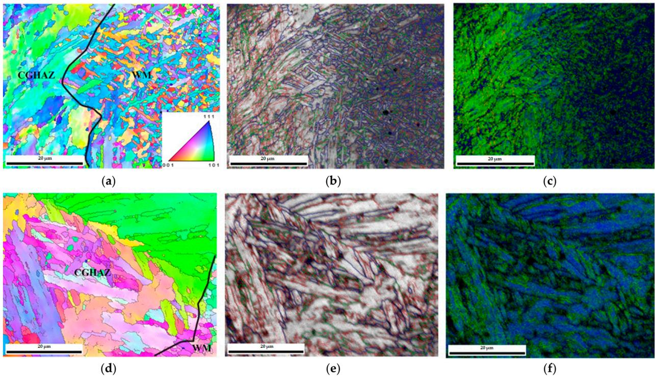
**Figure 6.** EBSD analysis of pre-fabricated crack tips under two heat inputs: (a–c) IPF map, size-angle grain boundary distribution map and KAM map for ultra-low heat input; (d–f) IPF map, size-angle grain boundary distribution map and KAM map for conventional heat input.
