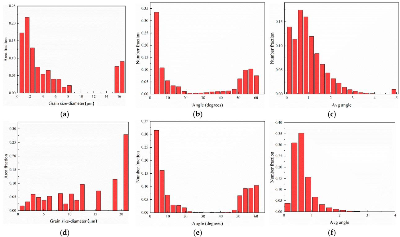
**Figure 7.** (a,d) Grain size, (b,e) size-angle grain boundary and (c,f) KAM distribution for ultra-low and conventional heat input, respectively.
