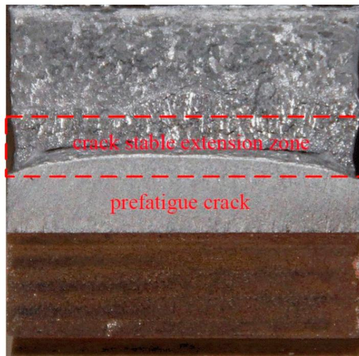
**Figure 8.** Location of the cloud image analysis of the fracture front of the prefabricated fatigue crack.
