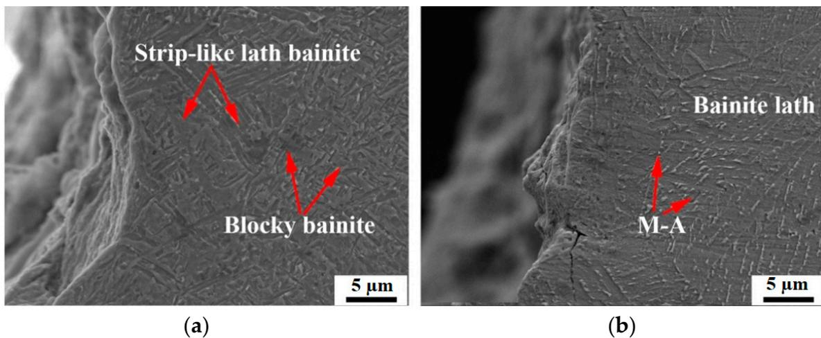
**Figure 5.** SEM microstructure at prefabricated fatigue crack tips using two heat inputs: (a) ultra-low heat input; (b) conventional heat input.
