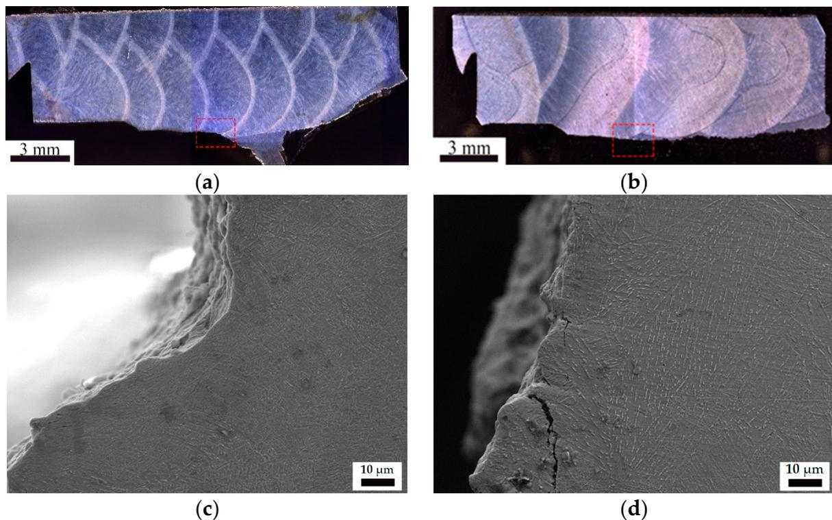
**Figure 4.** Optical microscope image of crack propagation path and SEM microstructure of plastic crack initiation position in CTOD test. (a,c) Ultra-low heat input; (b,d) conventional heat input.
