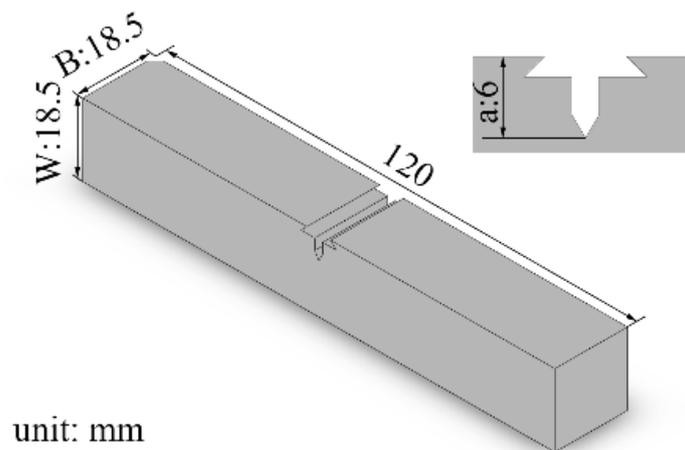
**Figure 3.** Description of prepared notch form of CTOD fracture toughness specimen (W: wall thickness of the steel pipe; a: depth of prepared notch).
