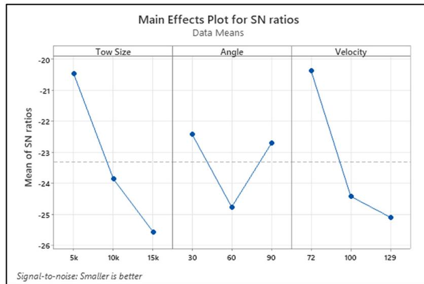
Figure 4. Main effect plot of the S/N ratio for erosion rate.
