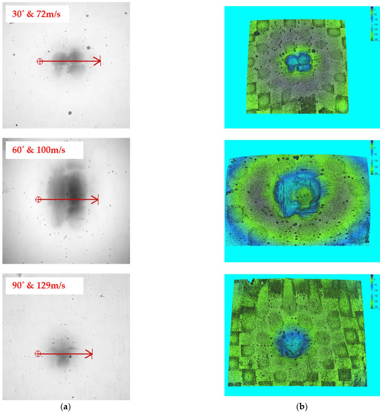
Figure 8. Eroded surface view for 5k samples: (a) microscopic view and (b) 3D surface profilometer image.
