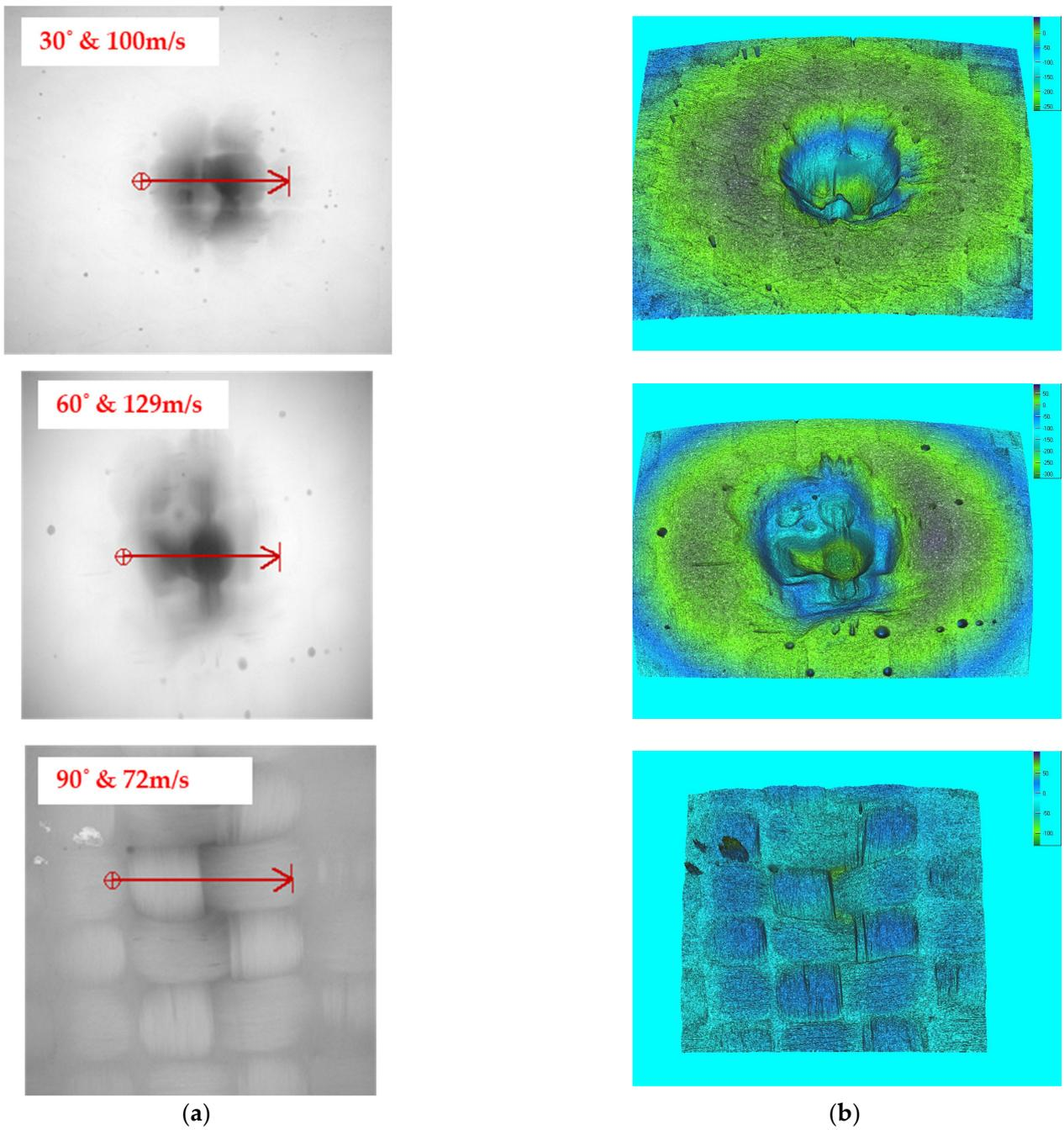
**Figure 9.** Eroded surface view for 10k samples: (a) microscopic view and (b) 3D surface profilometer image.
