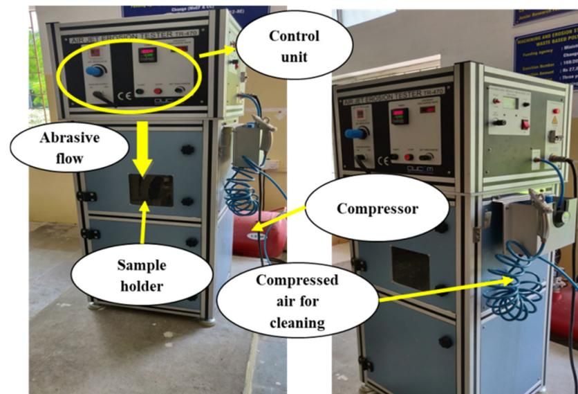
Figure 2. Erosion test facility.
