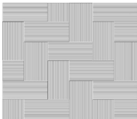
**Figure 1.** Representation diagram of  $2 \times 2$  twill weave pattern.
