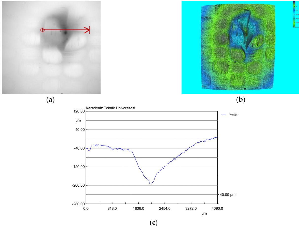
**Figure 7.** Surface of the eroded sample (Tow = 10k, Angle = 90 degrees, Velocity = 129 m/s), surface topography: (a) microscopic view, (b) 3D surface profilometer image, and (c) surface profile.
