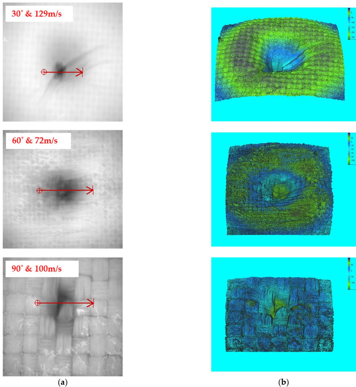
**Figure 10.** Eroded surface view for 15k samples: (a) microscopic view and (b) 3D surface profilometer image.
