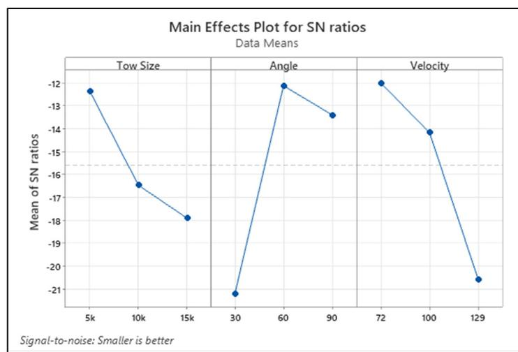
Figure 6. Main effect plot of S/N ratio for  $R_a$ .
