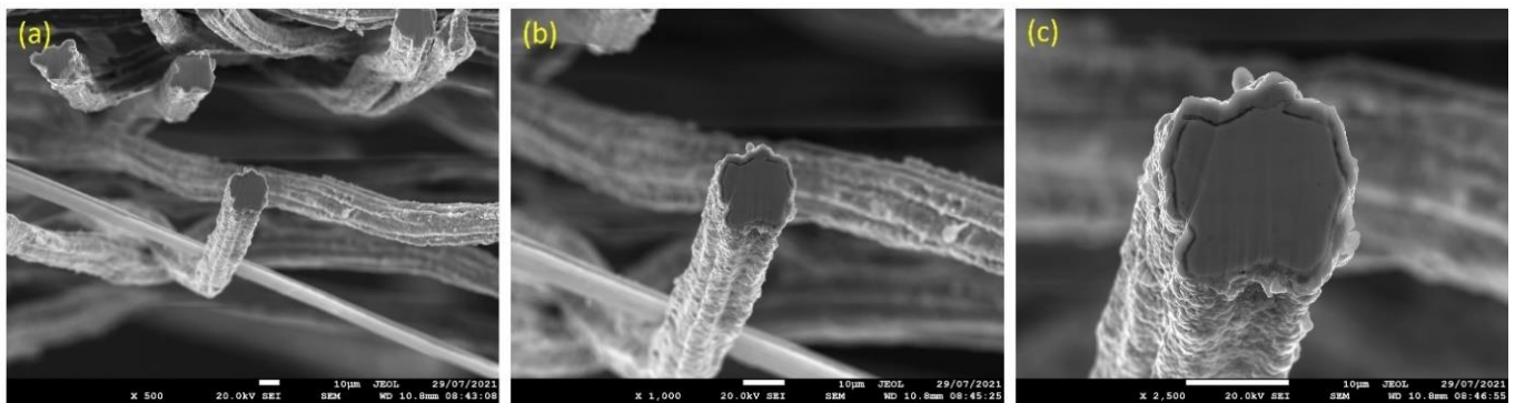
Figure 6. SEM micrographs of cross section of 12 \mu\text{m} FeCrAl fibers, after one MSHT cycle, at different magnifications: (a) \times 500 , (b) \times 1000 , and (c) \times 2500 .
