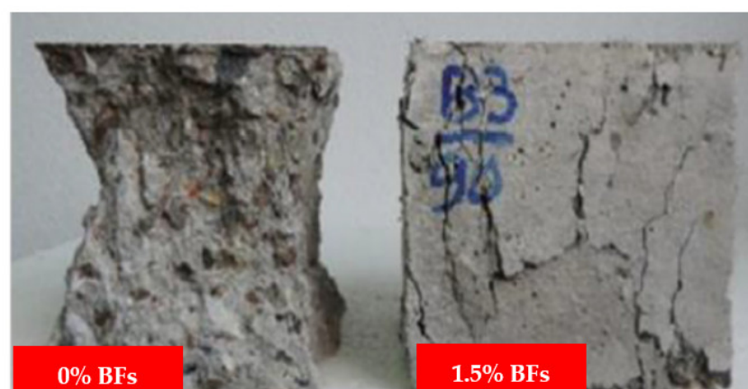
Figure 7. Compressive Failure Modes [50] with Elsevier permission.
