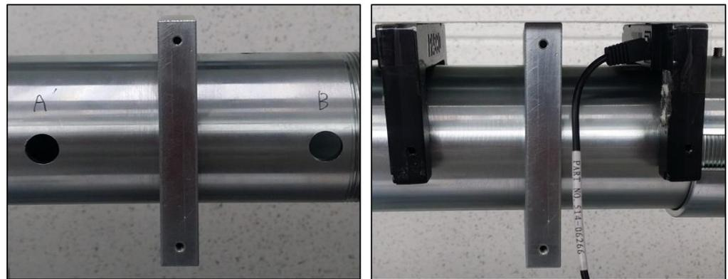
Figure 22. Photogate installed on the SHPB apparatus.
