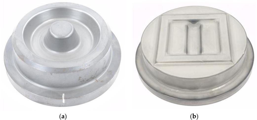
**Figure 6.** Selected forging die geometries for the laboratory validation processes: (a) Type 1 for further validation of the H11 base material data set, (b) Type 2 for the validation of the material data of the nitriding profile.
