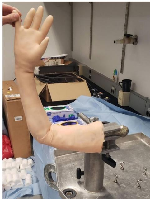
**Figure 8.** Photograph showing our phantom mounted in a vice to replicate a stationary patient in preparation for inducing traction.
