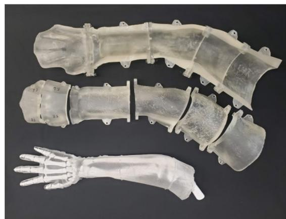
**Figure 6.** Photograph showing an unskinned phantom arm (bottom) beside its multi-piece casting mold (top) printed from FormLabs' SLA resin.
