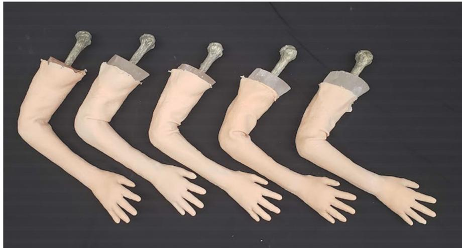
**Figure 7.** Photograph showing the replicability of full-arm phantoms, with slight variations seen in flesh and skin truncation along the humerus.
