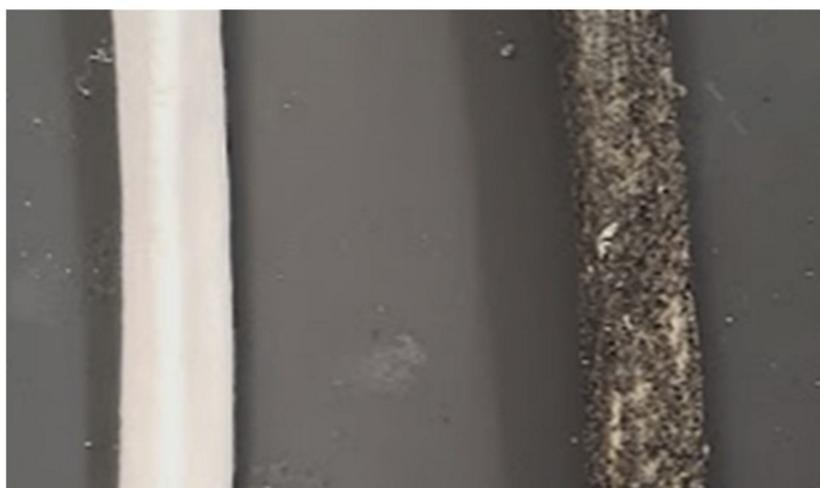
**Figure 2.** Photograph showing our periosteum-coated phantom bone segment (**right**) beside to a bare 3D print (**left**). Four individually cured layers produce a smooth sheath, improving behavior at joints, and controllable radiopacity.
