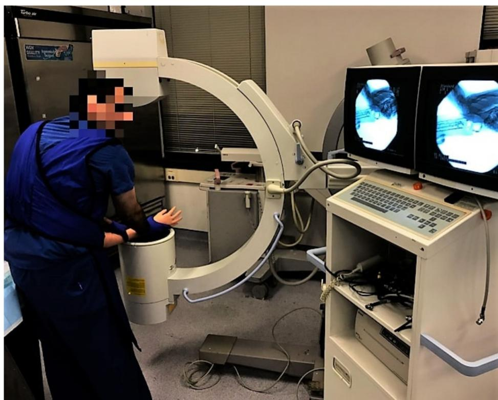
**Figure 9.** Photograph showing the examination of the phantom using C-arm fluoroscopy.
