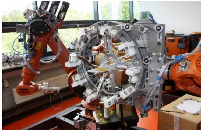
**Figure 2.** Robotized winding by using hybrid tapes (developed at TUL).
