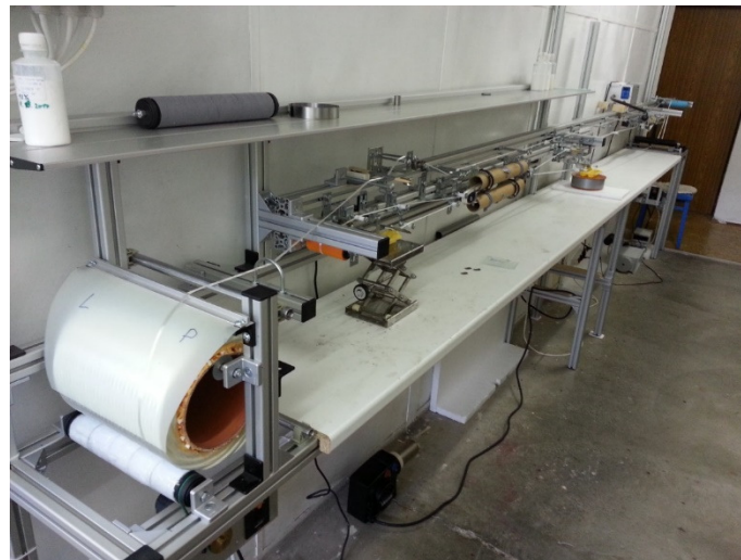
Figure 4. Semi-operating device for preparing a prepreg (© Global Science Press) [20].
