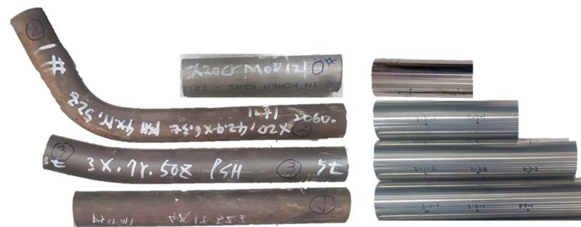
Figure 3. Boiler tube original samples (left) and after processing for ultrasonic measurement (right).
