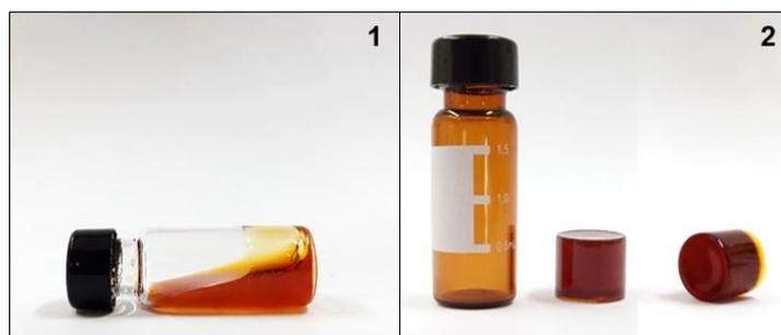
**Figure 10.** A sample based on the p-(GAT-co-GA)-14 copolymer before (1) and post-curing (2).
