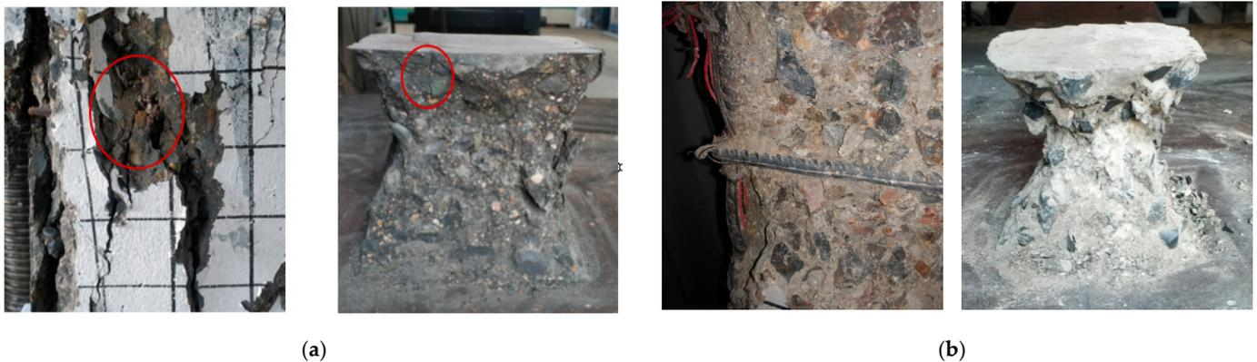
**Figure 7.** The aggregate failure mode of the specimens and blocks with different concrete strengths: (a) C100; (b) C50.
