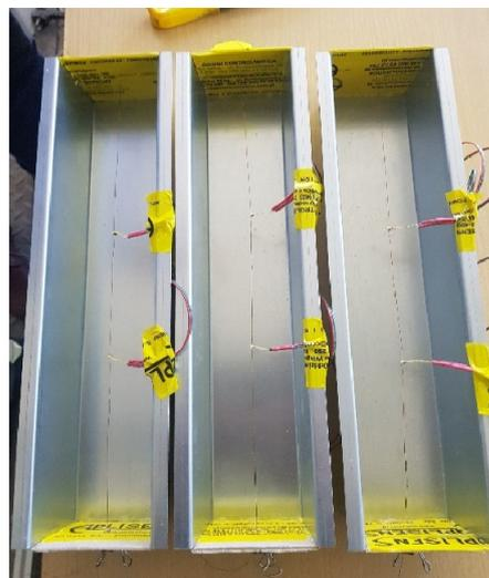
**Figure 1.** Gypsum molds with embedded wire.
