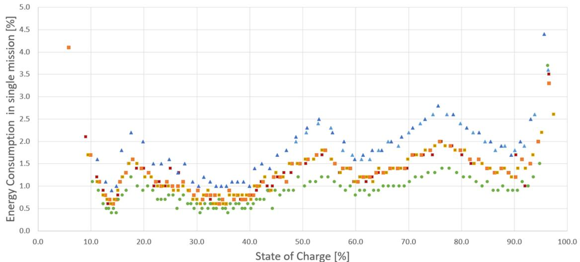
**Figure 4.** Battery discharge data for missions of different lengths.
