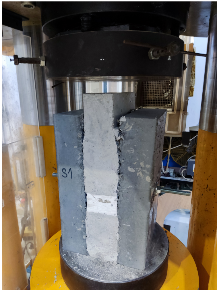
Figure 8. Sandwich sample in the hydraulic loading machine after testing.
