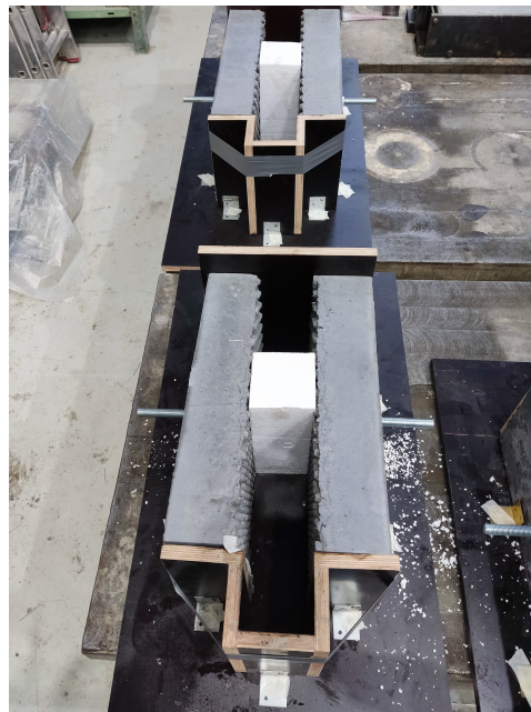
Figure 4. Sandwich samples prepared to be filled with NSC between two UHPC parts.
