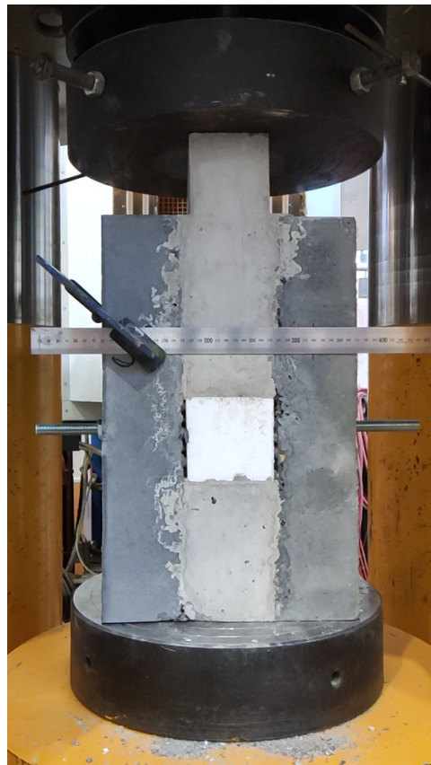
Figure 5. Sandwich sample prepared to be tested in hydraulic loading machine. The gauge is used to determine the formation of the crack.
