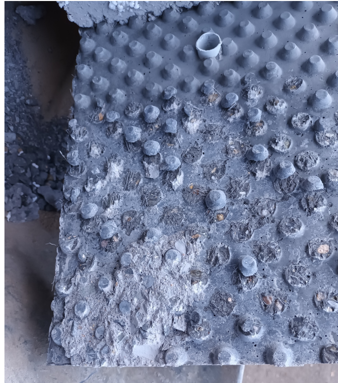
Figure 10. In the specimen, the buttons were sheared off in most of the area, but in some parts crack occurred in the filling concrete.
