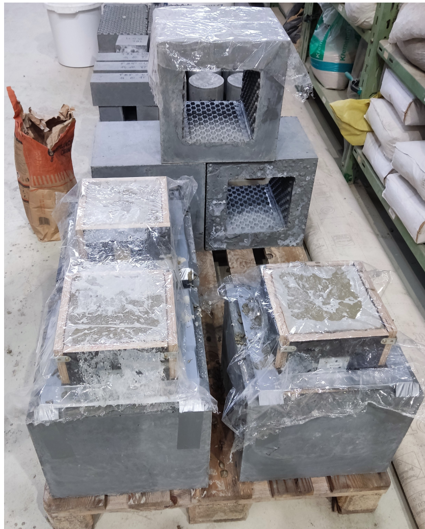
Figure 7. In the front section are box samples for testing of the interaction between UHPC and NSC1; behind them are parts of samples made from UHPC with buttons on the inner surface prepared to be filled with NSC2 with FBC-TB.
