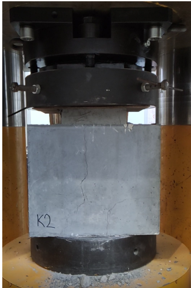
Figure 9. Box sample in the hydraulic loading machine during testing after the crack occurred.
