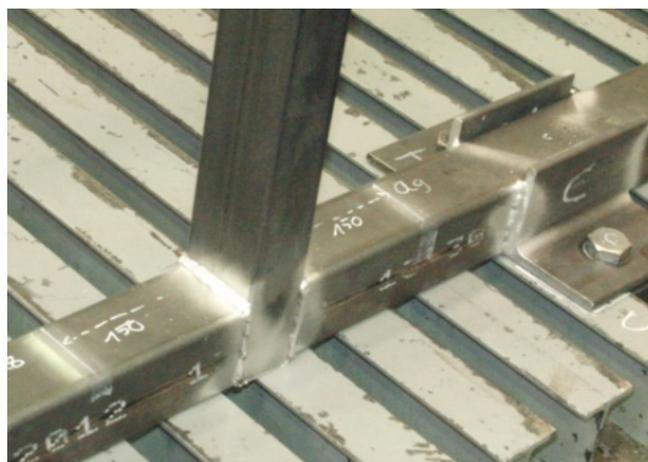
**Figure 5.** Clamping weld details.
