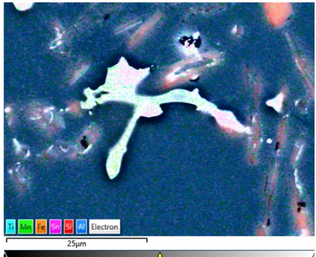
Figure 16. SEM-EDS layered image—AlSi10Sn1.7 alloy.
