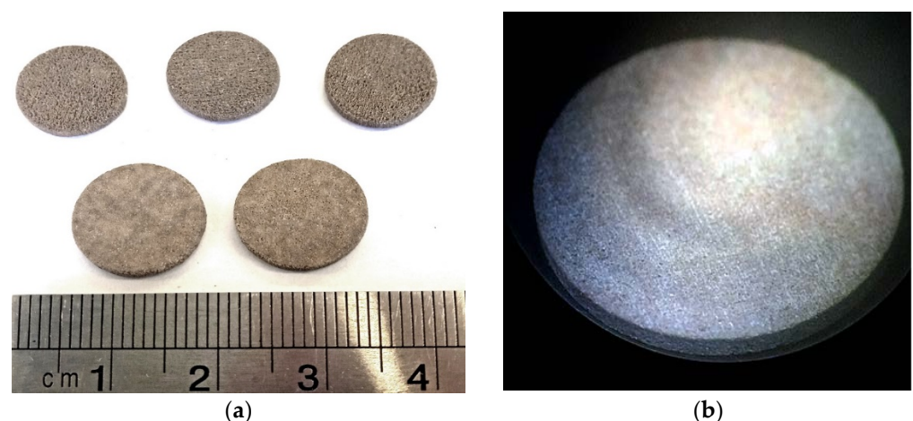
Figure 8. Images of BCZT samples manufactured by BJ for the functional property measurements: (a) samples after sintering; (b) samples after silver electrode coating.
