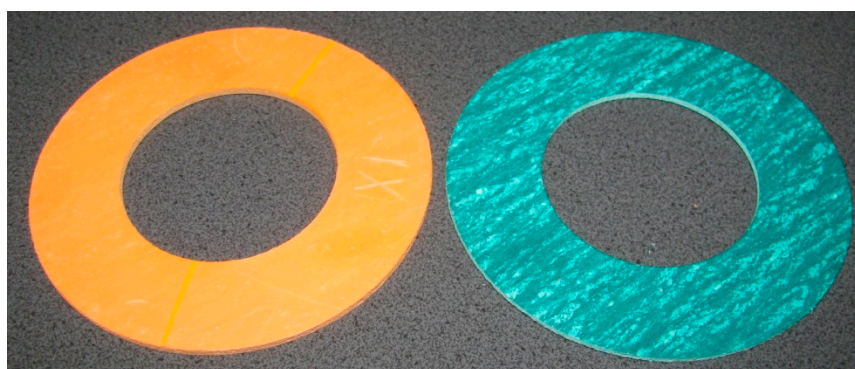
Figure 2. View of the tested gaskets; AFM—on the left, AFO—on the right.
