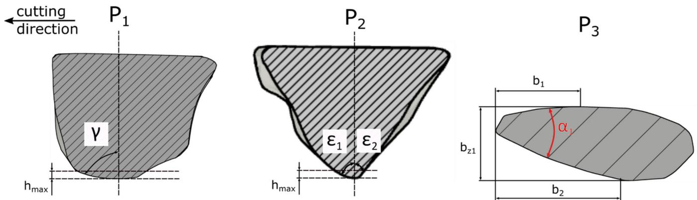
**Figure 5.** Geometrical properties of abrasive grain ZS1.
