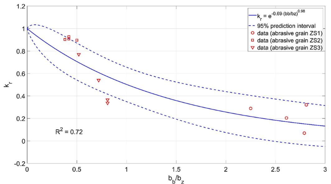
**Figure 20.** Influence of the coefficient  $b_b / b_z$  of the abrasive grain on the material removal efficiency  $k_r$ .
