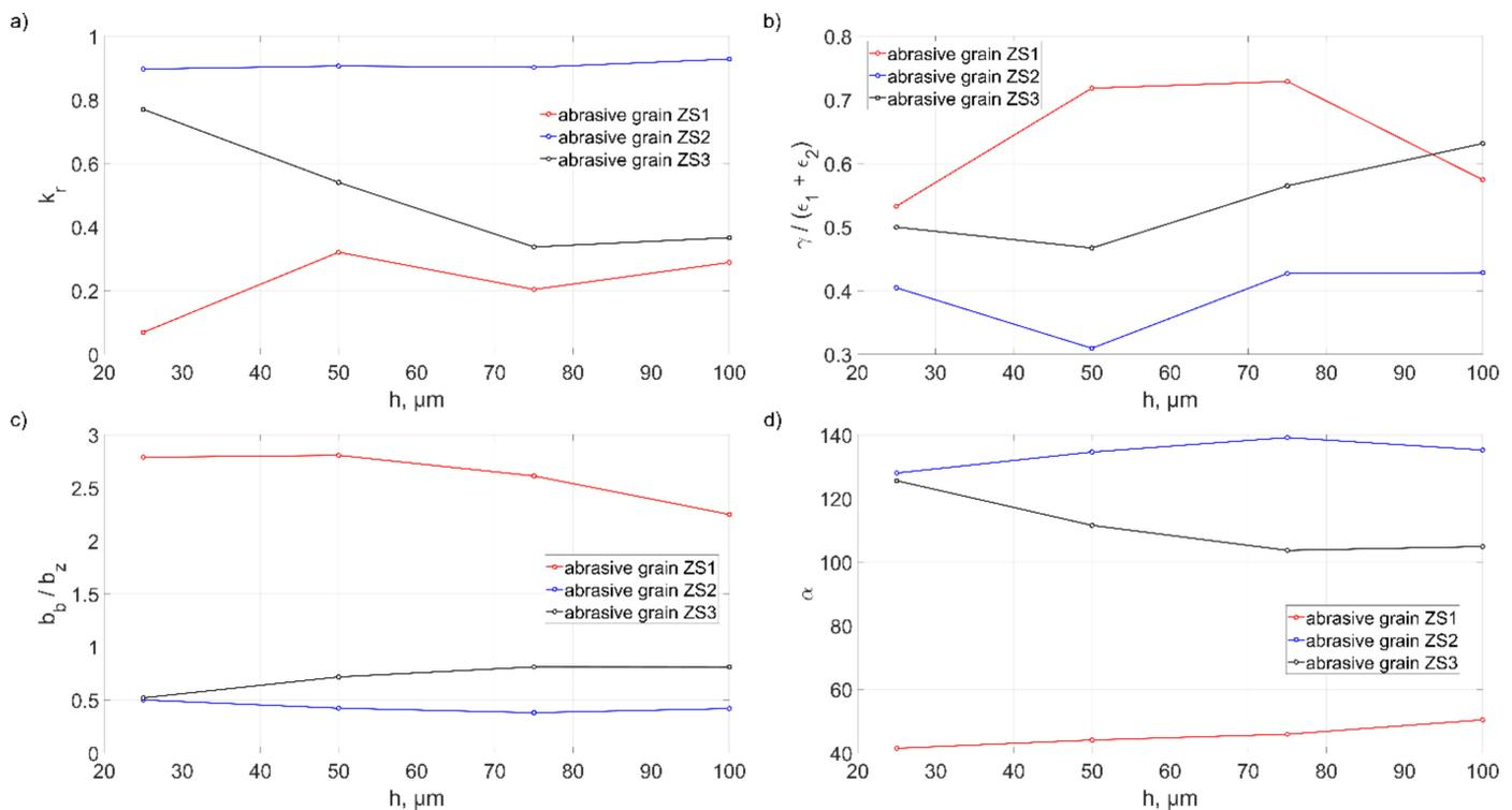
**Figure 18.** Influence of cutting depth  $h$  of abrasive grains with different geometry on: (a) the volumetric material removal coefficient  $k_r$ , (b) the coefficient  $\gamma/\varepsilon$ , (c) the coefficient  $b_b/b_z$ , (d) the opening angle  $\alpha$ .
