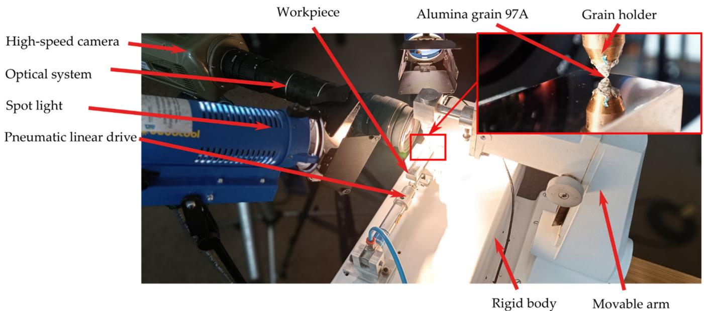
**Figure 3.** General view of the test stand for scratch tests.
