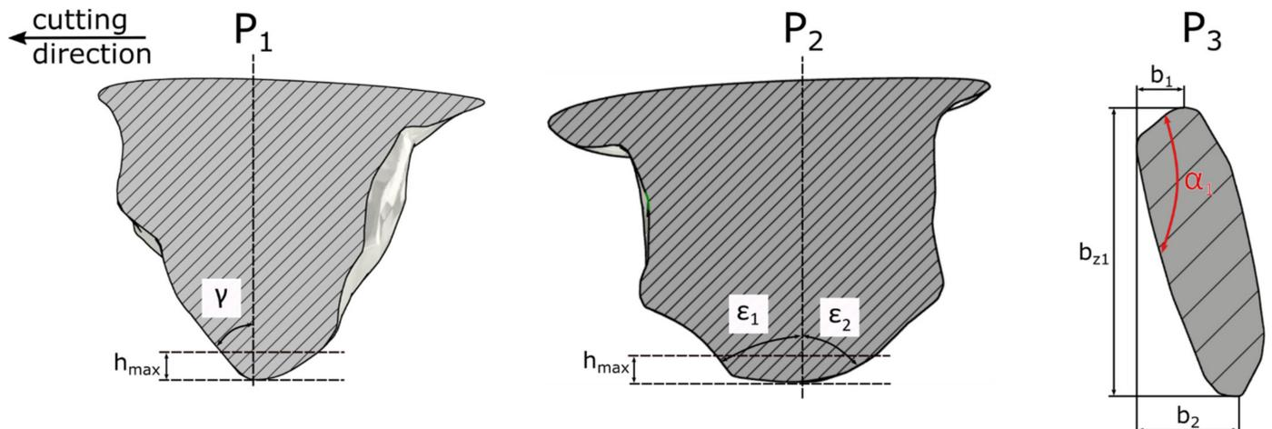
**Figure 6.** Geometrical properties of abrasive grain ZS2.
