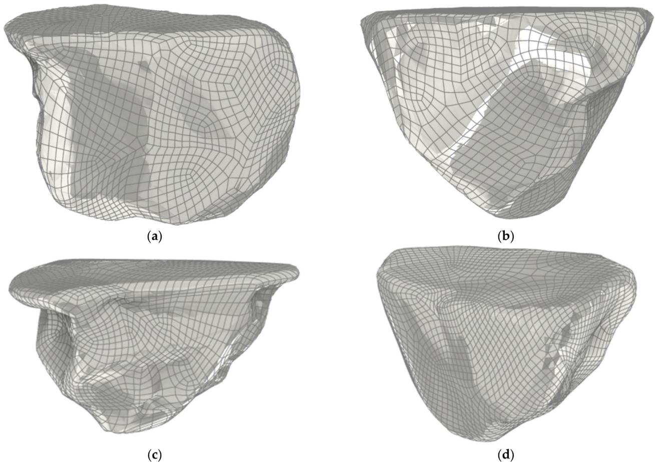
**Figure 1.** Alumina grains 97A with size F20, applied for numerical model validation (a) and numerical simulations (b–d).
