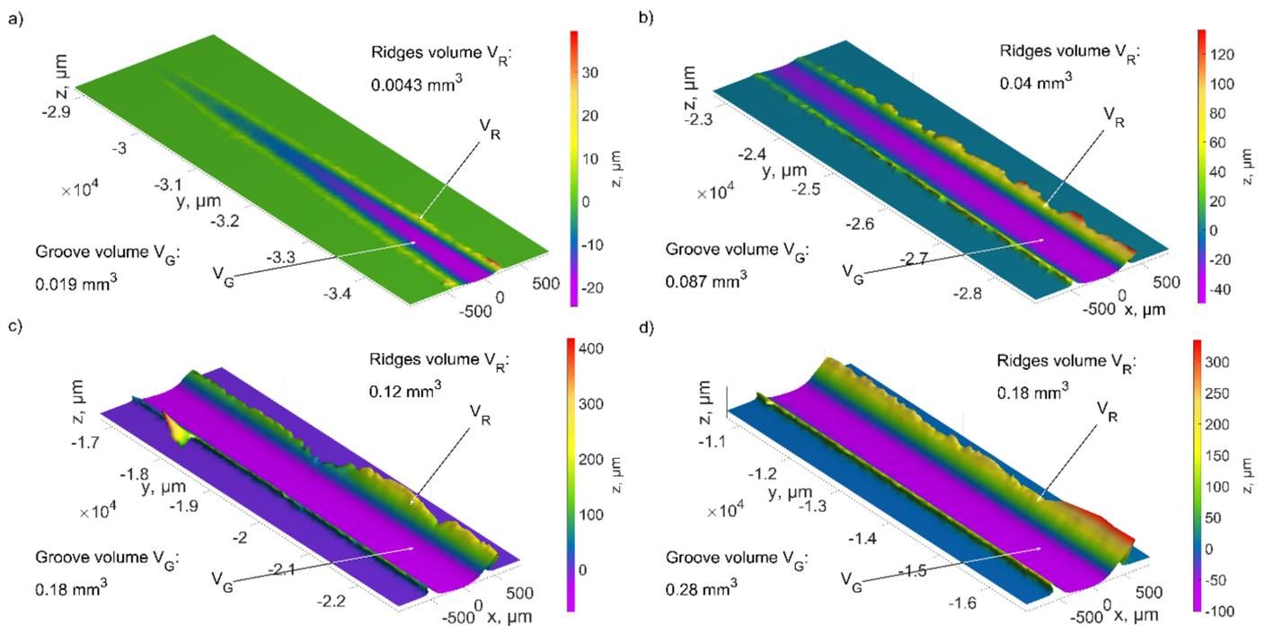
**Figure 17.** The results of the scratch volume and pile ups after the ZS3 grain cutting process for the depth of cut: (a) from 0 to 25  $\mu\text{m}$ , (b) from 25  $\mu\text{m}$  to 50  $\mu\text{m}$ , (c) from 50  $\mu\text{m}$  to 75  $\mu\text{m}$ , (d) 75  $\mu\text{m}$  to 100  $\mu\text{m}$ .
