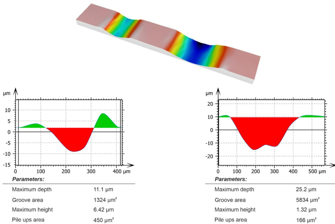
**Figure 10.** Cross-sections of the scratches—numerical results.
