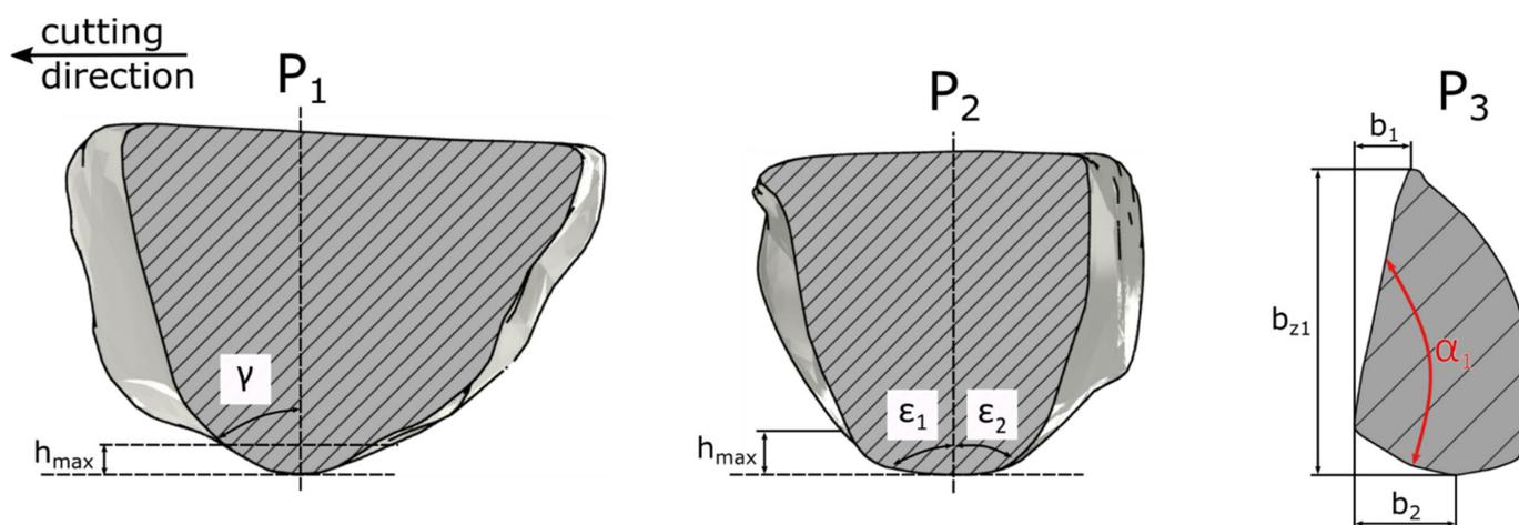
Figure 7. Geometrical properties of the abrasive grain ZS3.
