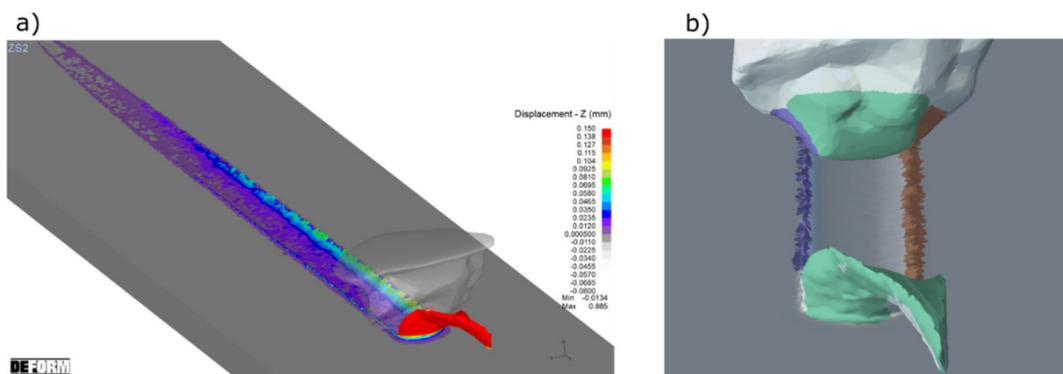
**Figure 14.** The results of a computer simulation of the cutting process with ZS2 grain (a) and the colored areas which caused the plastic flows of the processed material (b).
