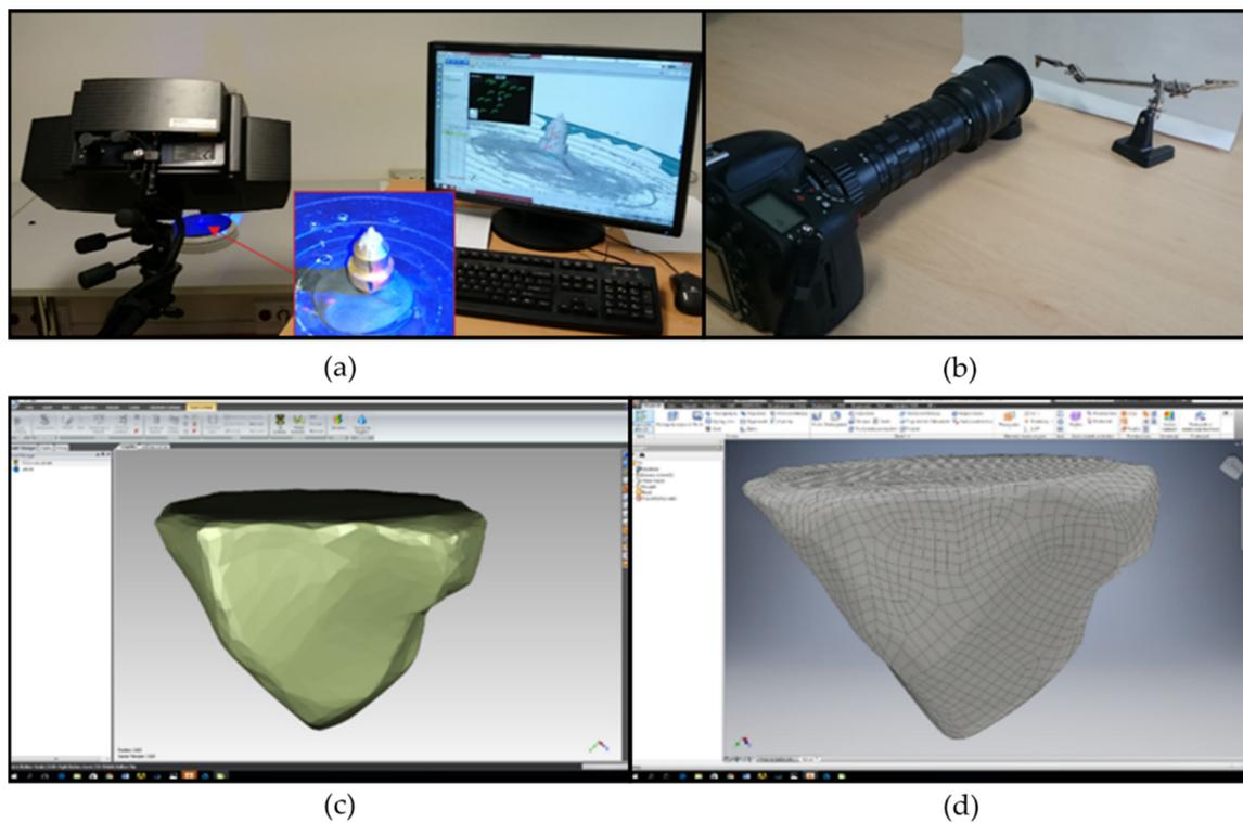
**Figure 2.** Methodology of abrasive grains shape reconstruction: (a) 3D scanning, (b) taking the macrotopography, (c) processing of the point clouds in the Geomagic software, (d) analysis of the geometric properties in Autodesk Inventor software.
