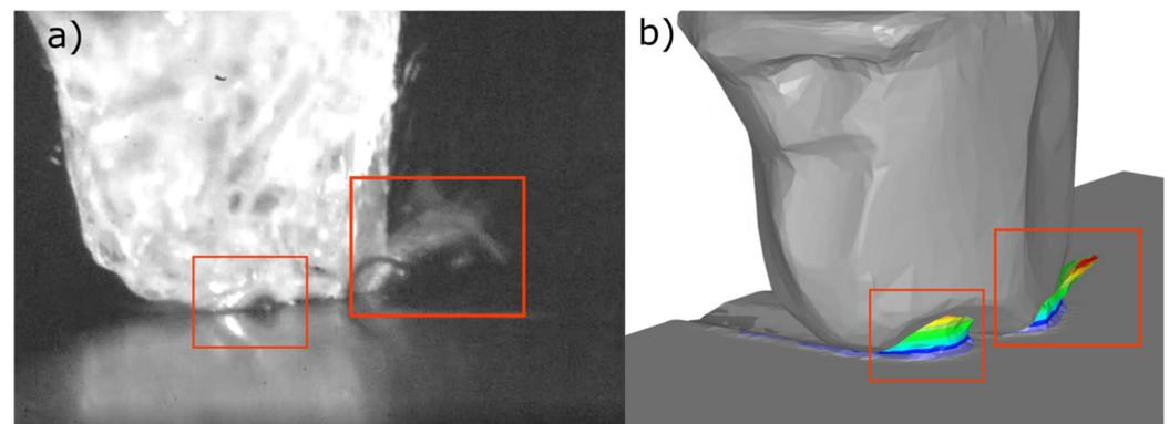
**Figure 11.** Frame from the high-speed camera (a) and the simulation process (b) as a part of the validation method.
