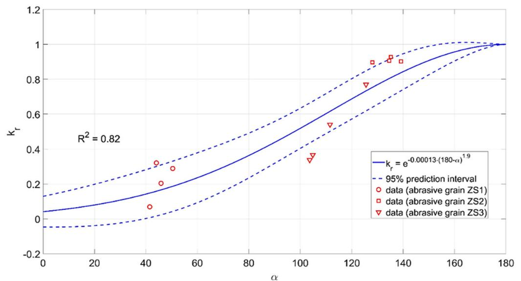
**Figure 21.** Influence of the opening angle  $\alpha$  of the abrasive grain on the material removal efficiency  $k_r$ .
