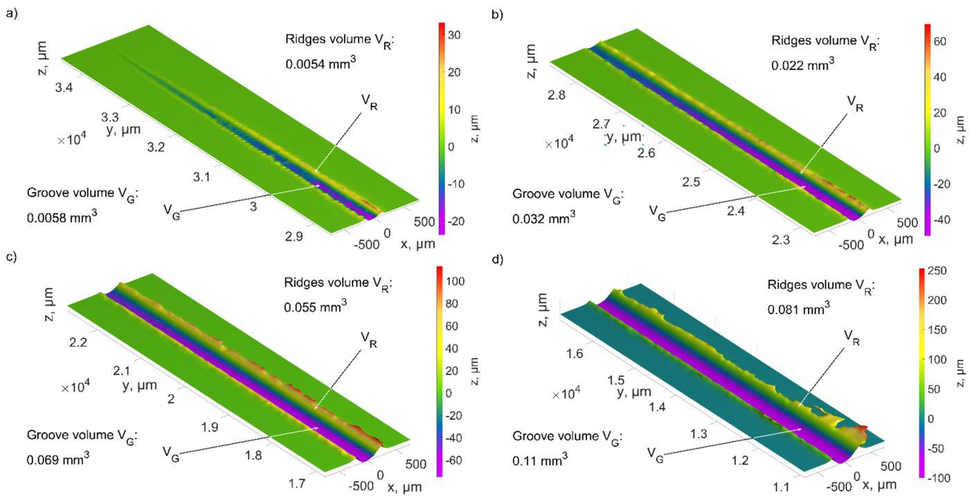
**Figure 13.** The values of the scratch volume and pile ups after the ZS1 grain cutting process for the depth of cut: (a) from 0 to 25  $\mu\text{m}$ , (b) from 25  $\mu\text{m}$  to 50  $\mu\text{m}$ , (c) from 50  $\mu\text{m}$  to 75  $\mu\text{m}$ , (d) 75  $\mu\text{m}$  to 100  $\mu\text{m}$ .
