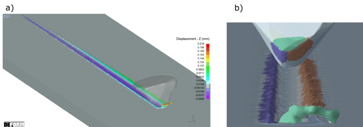
**Figure 12.** The results of the computer simulation of the cutting process with ZS1 grain (a) and the colored areas which caused the plastic flows of the processed material (b).
