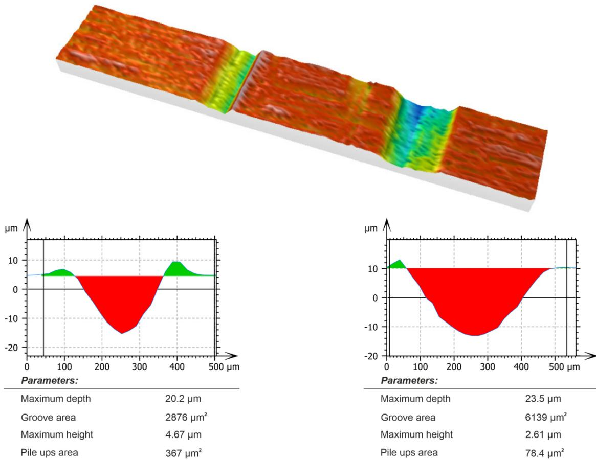
**Figure 9.** Cross-sections of the scratches—experimental results.
