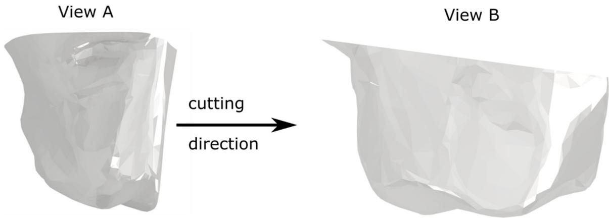
**Figure 8.** The cutting grain used for experimental validation of the numerical simulations.
