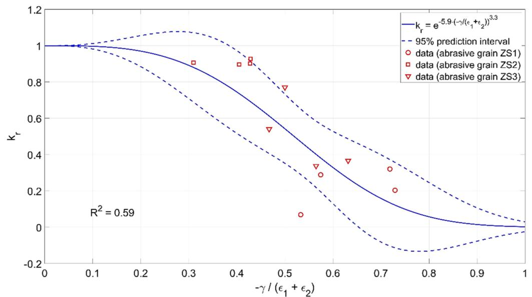
**Figure 19.** Influence of the ratio of the rake angle  $\gamma$  to the apex angle  $\epsilon$  of the abrasive grain on the material removal efficiency  $k_r$ .
