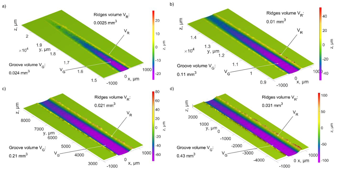
**Figure 15.** The results of the scratch volume and pile-ups after the ZS2 grain cutting process for the depth of cut: (a) from 0 to 25  $\mu\text{m}$ , (b) from 25  $\mu\text{m}$  to 50  $\mu\text{m}$ , (c) from 50  $\mu\text{m}$  to 75  $\mu\text{m}$ , (d) 75  $\mu\text{m}$  to 100  $\mu\text{m}$ .
