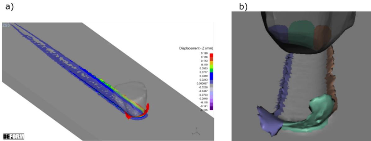
**Figure 16.** The results of a computer simulation of the cutting process with ZS3 grain (a) and the colored areas which caused the plastic flows of the processed material (b).
