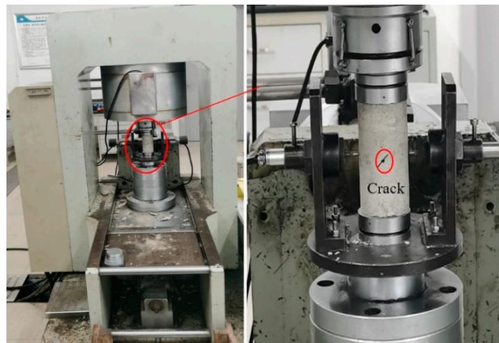
**Figure 1.** RMT-150B electro-hydraulic servo-controlled test machine system.
