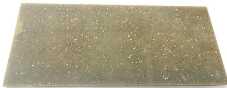
Figure 1. The sample prepared for hardness tests, R10, dimensions 300 \times 100 .
